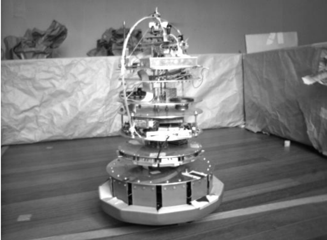
Figure 2: Typical robotic agent used in behavior-oriented AI experiments. The robot has a ring of infrared sensors and a ring of bumper sensors. It has additional light sensors and microphones. There is a translational motor for forward/backward movement and a rotational motor for turning left or right. The agent has a central PC-like processor and dedicated hardware for signal processing and interdevice communication.
