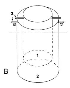
Fig 1. A) Schematic diagram of the incubation system used in the food fluctuation experiments. (1) 15 l plastic container, (2) egg-laying chambers, (3) peristaltic pump, (4) flow regulator. B) Digram of an egg-laying chamber. (1) 200 $\mu$ m nitex-mesh, (2) 40  $\mu$ m nitex-mesh, (3) hanging system.
