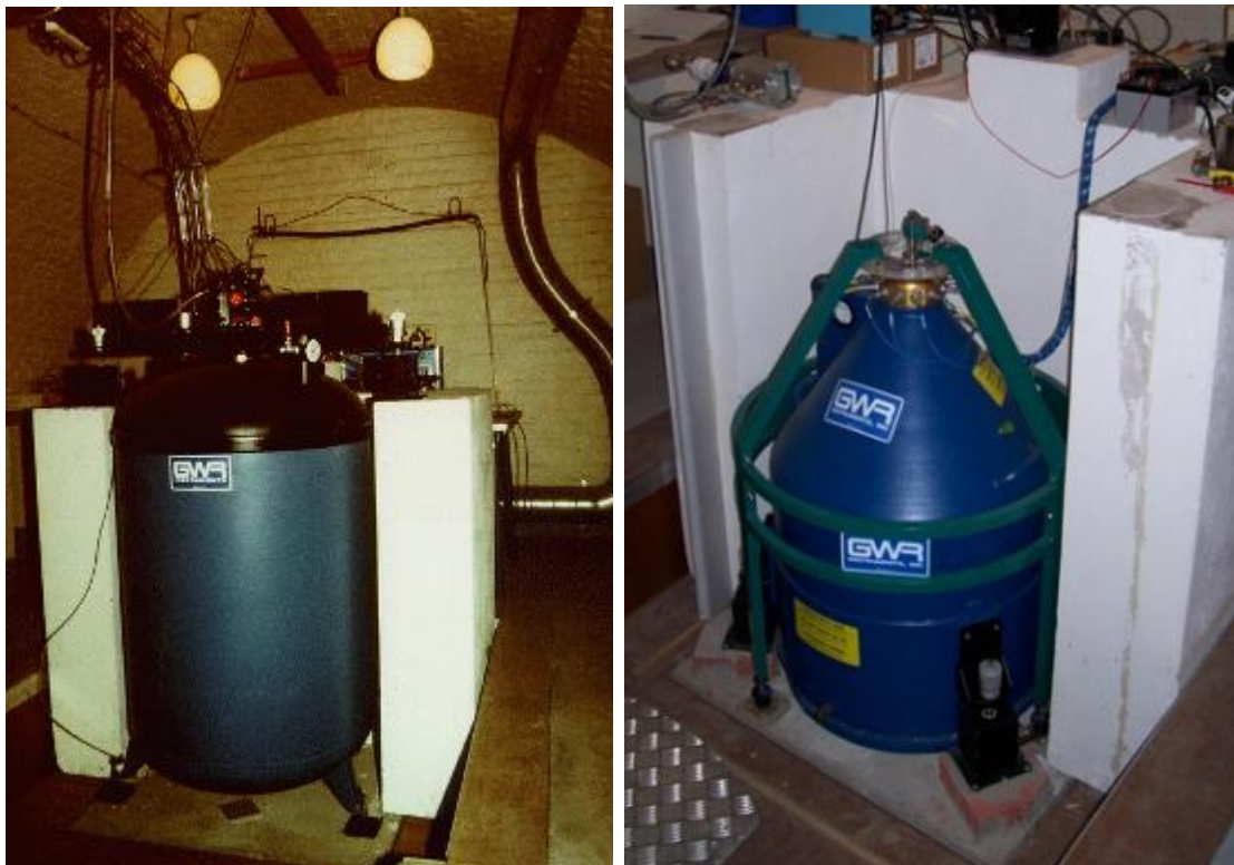
Fig. 3.10: Superconducting gravimeters installed at the J9 Observatory. Left one: TT70 model (T005). Right one: compact SG model (C026).
