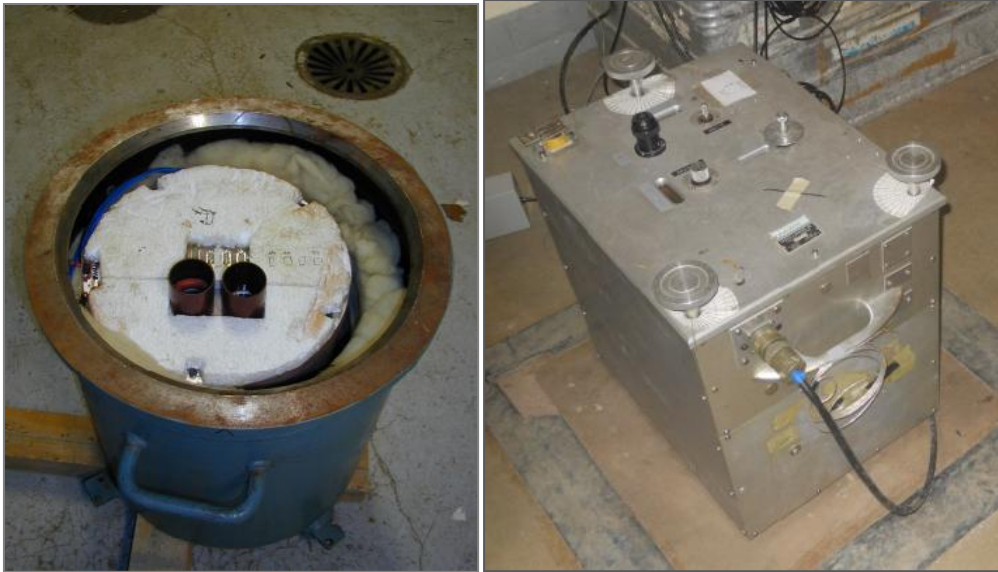
Fig 3.7: Pictures of the isolated boxes where the spring gravimeters L&R ET005 (left picture) and the L&R ET11 (right picture) were installed at J9 Observatory.
