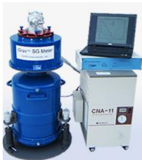
Fig. 2.2.8: New \mu\text{Grav} superconducting gravimeter, manufactured by GWR Instruments (extracted from GWR website, http://www.gwrinstruments.com ).
