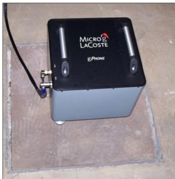
Fig 3.8: Spring gravimeter Microg-LaCoste gPhone 054 owned by IGN-Spain, installed at J9 Observatory between 2008 and 2009.
