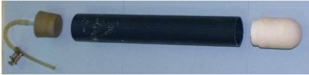
Ceramic suction cup (homemade; 15 €)
