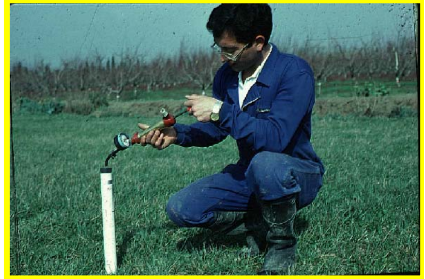
Ceramic suction cup (homemade; 15 €)
