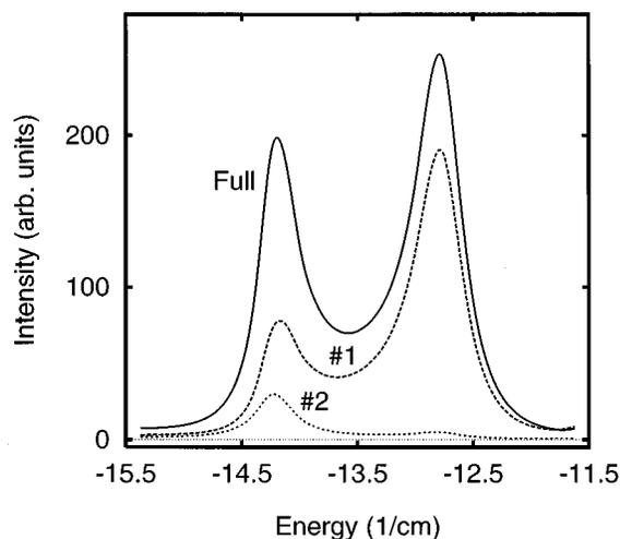
FIG. 1. Solid line: total cross section (in arbitrary units) as a function of energy (in  $\text{cm}^{-1}$ ) for the  $v_0=45$  level (“full” calculation). Dashed line (#1): Same for the artificial Franck–Condon factors scheme of Eq. (3.2). Dotted line (#2): Same for the artificial Franck–Condon factors scheme of Eq. (3.3). Energy is referred to the  $\text{Br}_2(B, v=45)$  level.
