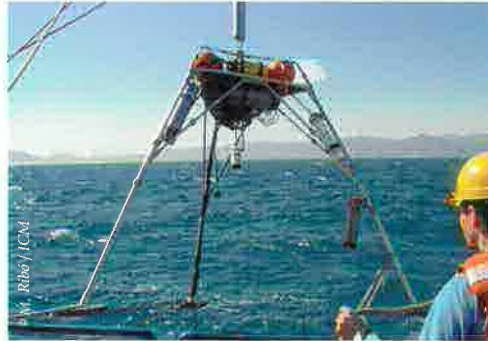
Benthic tripod for the monitoring of sediment transport near the sea bottom.
