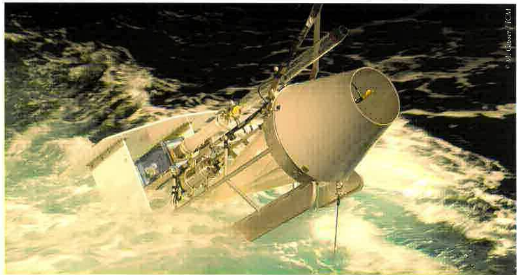
A Longhurst Hardy Plankton Recorder: a device with two fishing nets for collecting plankton of different sizes simultaneously at different depths.
