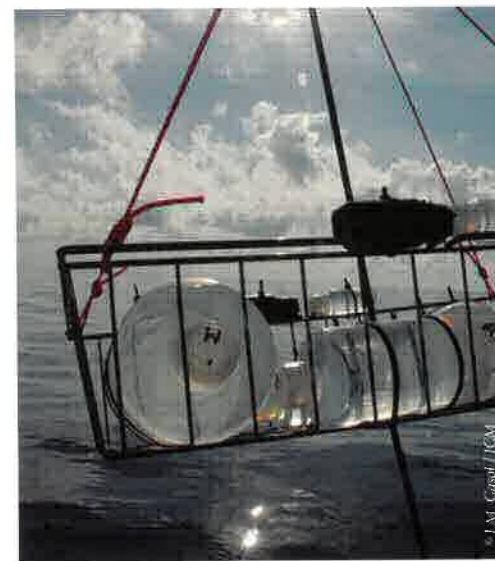
Experiment to determine the effect of light on the metabolism of microorganisms, using bottles with different transparencies.
