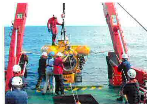
Deployment of the submersible JAGO to study the seabed life up to 500 metres depth.
