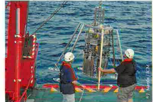
Taking aboard the multicore, a device used to study sediments and particle fluxes.
