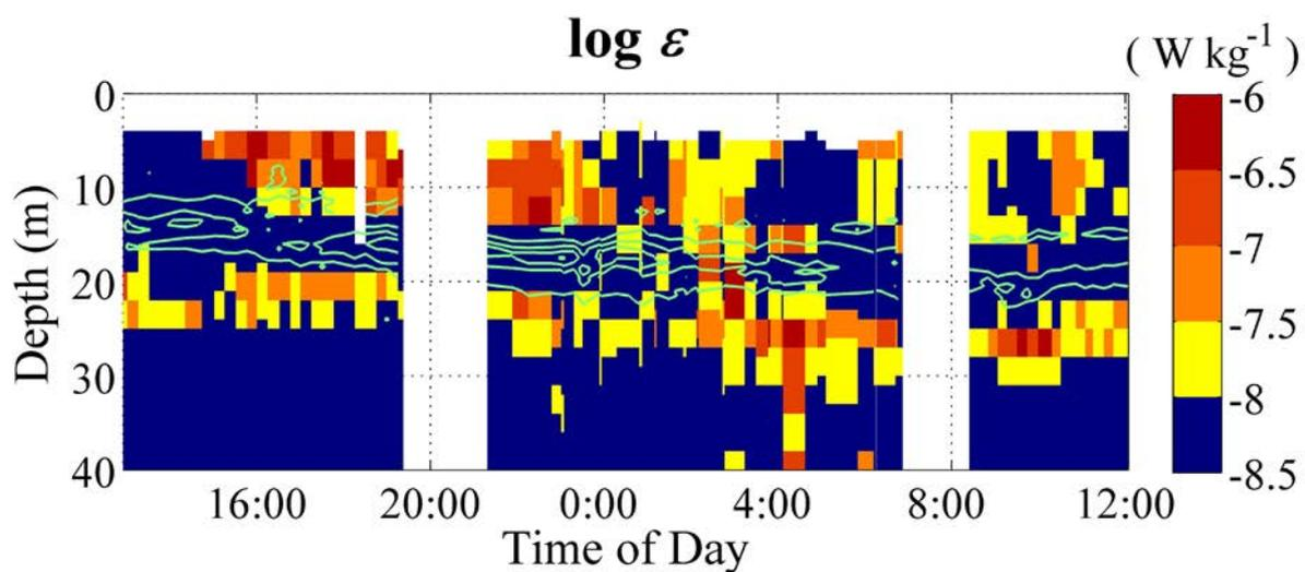
**Figure 3.** The distribution of the rate of the kinetic energy dissipation ( $\text{W kg}^{-1}$ ) is depicted with contours of chlorophyll concentration ( $1.5\text{--}2.8 \mu\text{g}\cdot\text{L}^{-1}$  range). The local peak in chlorophyll clearly appeared in the low dissipation rate region. All data were measured by TurboMAP-Ln (redrawn from Yamazaki et al. 2010).
