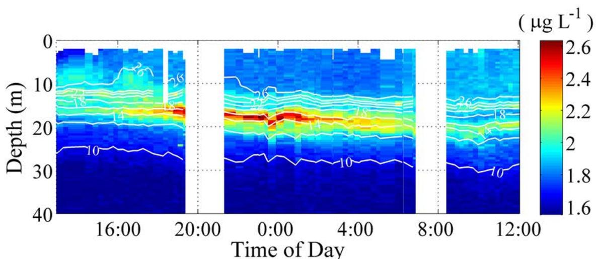
**Figure 4.** The chlorophyll distribution ( $\mu\text{g L}^{-1}$ ) and temperature structure (contoured in  $^{\circ}\text{C}$ ) measured over the survey period. A pronounced chlorophyll peak layer appeared in the strongly stratified water region of the water column where the temperature dropped from 18 to  $14^{\circ}\text{C}$ . All data were obtained from TurboMAP-L deployed at 15 minute intervals (redrawn from Yamazaki et al. 2010).
