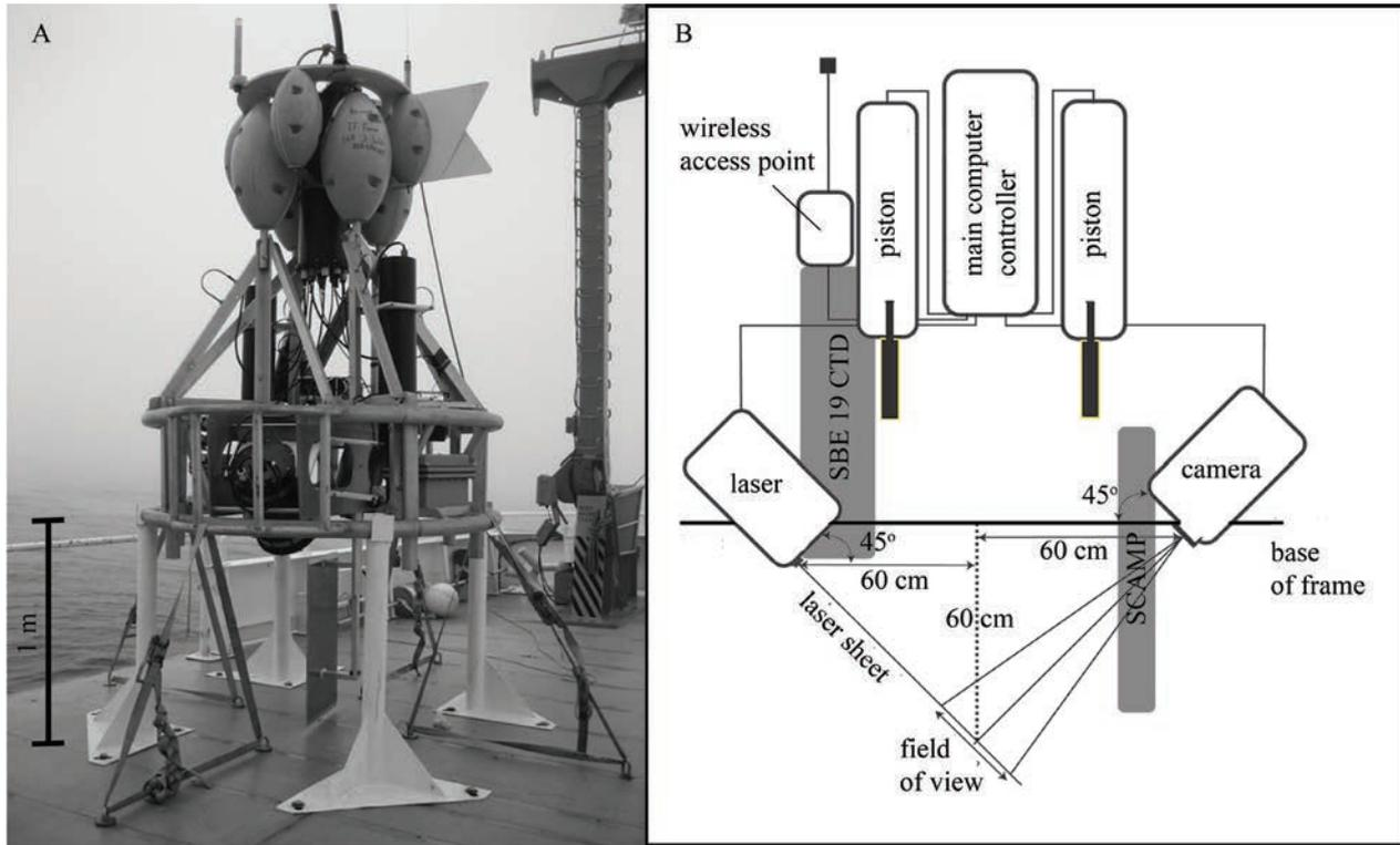
**Figure 6.** (a) The FIDO-Phi on deck of the R/V Wecoma. (b) Schematic of the FIDO-Phi system showing the camera and laser housings and the region where the laser sheet is imaged. The placement of the attached WET Star fluorometer and SCAMP are also shown (from Prairie et al. 2011, with permission from the editor).
