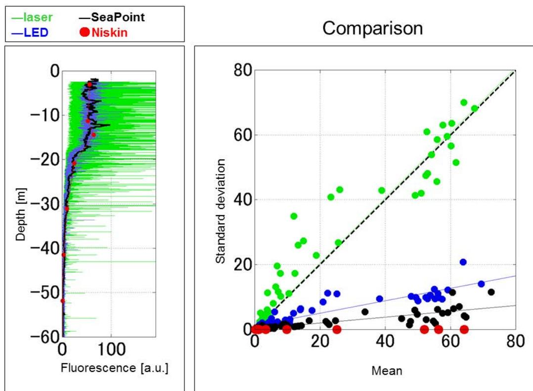
**Figure 1.** Fluorescence signals from laser probe and LED probe mounted on a microstructure profiler TurboMAP-L are plotted against depth. Also shown are signals from SeaPoint probe mounted on a conventional CTD as well as the water sample data from Niskin bottle. The corresponding mean and standard deviation for one-meter interval are shown in the right hand side.
