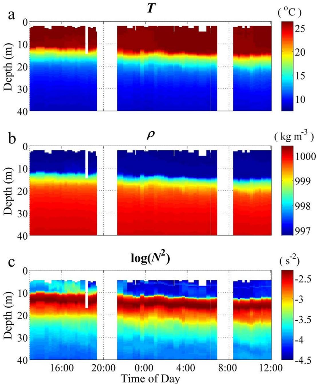
**Figure 2.** Distribution of (a) temperature, (b) density, and (c)  $\log_{10}$  of buoyancy frequency determined from TurboMAP-L profiling during the experiment. Profiles were obtained every 15 minutes. The surface mixed layer (epilimnion) is roughly 11 m at the beginning of the experiment and deepened slightly toward the end of the experiment (redrawn from Yamazaki et al. (2010)).
