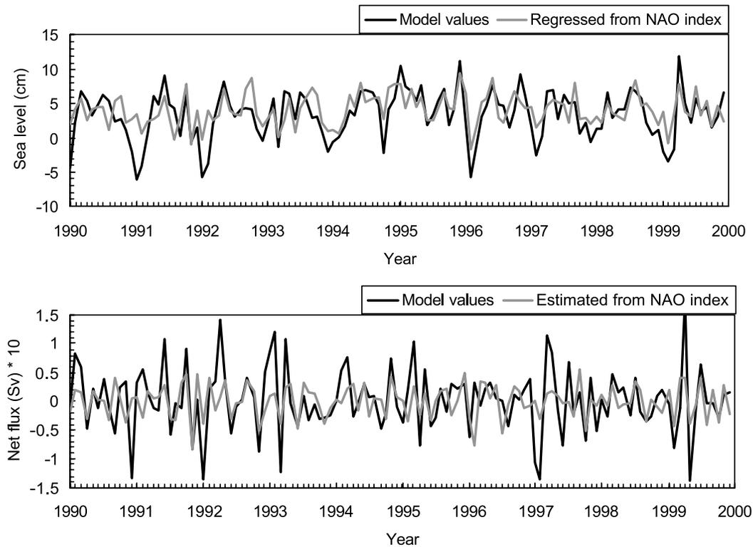
**Figure 8.** (top) Comparison between monthly mean sea level given by the model and the values regressed from the NAO index for the decade 1990–2000. (bottom) As in Figure 8 (top) but for the monthly mean flow through the Strait of Gibraltar.
