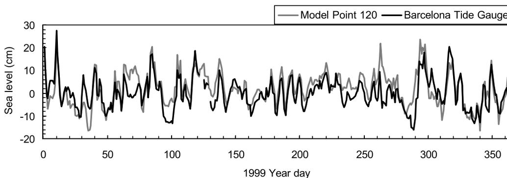
**Figure 1.** Sea level residuals from the Barcelona tide gauge ( $41^{\circ}21'01''\text{N}$ ,  $2^{\circ}9'41''\text{E}$ ) and model values at the closest grid point ( $41^{\circ}20'00''\text{N}$ ,  $2^{\circ}15'00''\text{E}$ ) during 1999.
