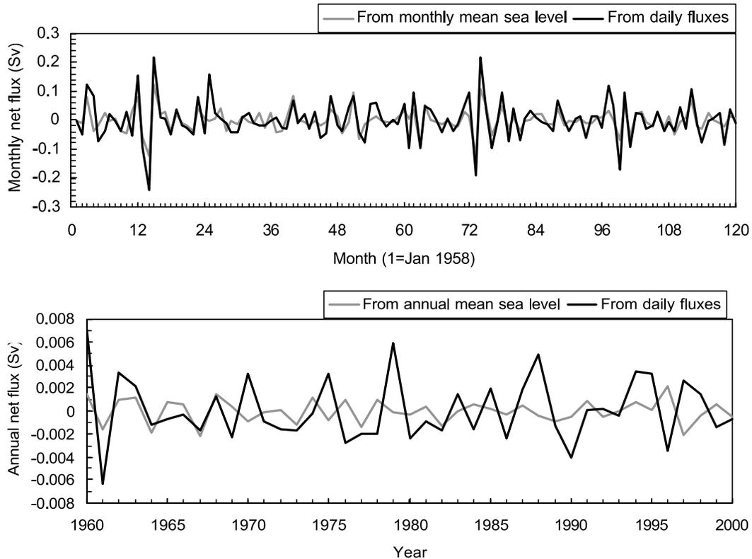
**Figure 3.** Comparison between the mean flow computed as the average of daily flow values and that computed from mean sea level values. (top) Monthly means (only the first 10 years of the modeled period have been plotted). (bottom) Annual means.
