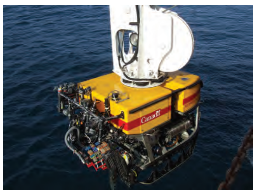
Above: CHONE scientists use ROPOS ("Remotely Operated Platform for Ocean Science"), an ROV, to conduct research on the ecology of hydrothermal vents, sponge reefs and cold-water corals, and begin pioneering work on cabled deep-sea observatories. Photo Credit: CSSF/ROPOS
