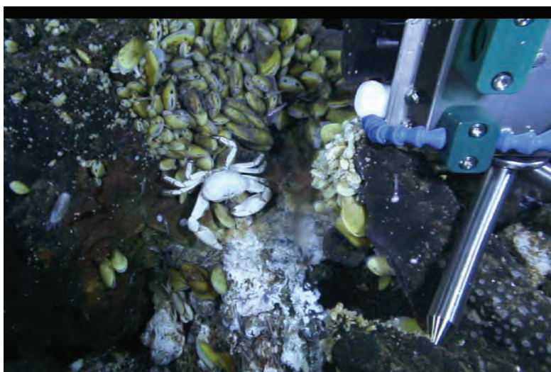
Above: the MoMAR observatory transmits one low-resolution image of the Bathymodiolus azoricus faunal assemblage that is being monitored on the Lucky Strike vent field along with related oxygen and temperature data. SMOOVE/Momarsat observatory 2010 (c) Ifremer.
