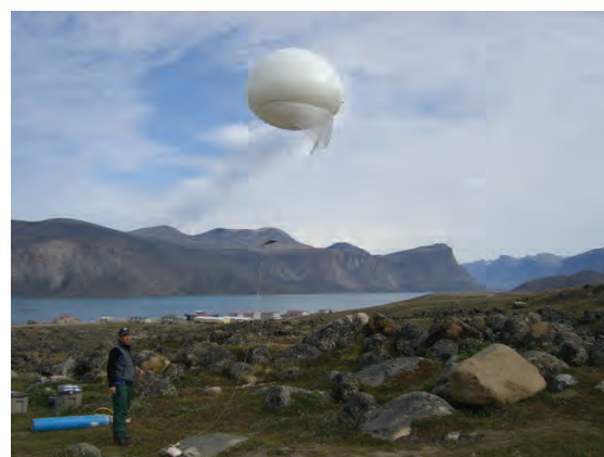
Above: Dalhousie University/CHONE researchers Jon Grant, Mike Dowd, and Jeff Barrell use a helium-inflated blimp as an aerial photography platform for studying the spatial patterning of intertidal landscapes. Pangnirtung, Baffin Island, Nunavut. Photo Credit: Jeff Barrell
