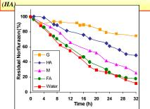
In general, the presence of the different soil components in suspension provoked a reduction in NFL photodegradation rate, due to the screen effect of soil particles and probably to the adsorption of NFL on these colloidal components. In all cases the rate of photodecomposition followed a first-order kinetic.
