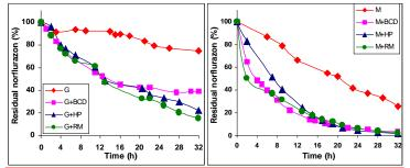
NFL photodegradation profiles in aqueous suspensions of montmorillonite (M) and goethite (G) in the presence of different CDs (BCD, HP and RM).
