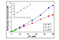
The increase in NFL solubility in the presence of the three cyclodextrins employed indicates the formation of inclusion complexes between the herbicide and the CDs. For the concentration used in photodegradation experiments (0.01M), linear increases up to 1.72, 4.46 and 4.95 fold in NFL solubility in aqueous solution were obtained using BCD, HP and RM, respectively.
