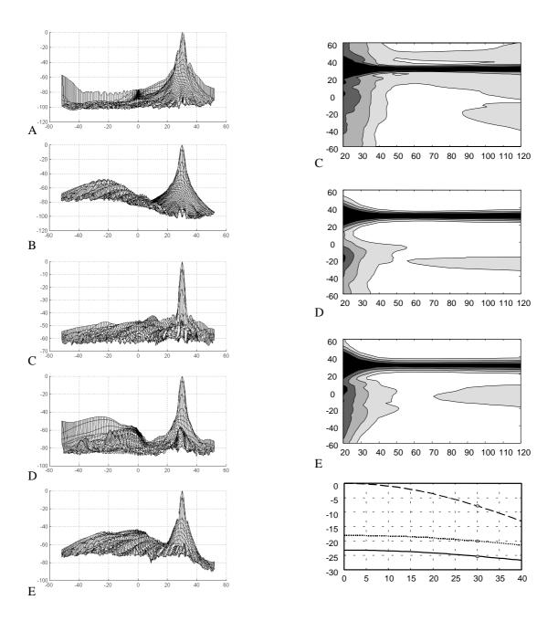
Figure 2. Beam profiles for a target point at  $(r=60\text{mm}, \theta=30^\circ, \phi=0^\circ)$  for the five array configurations: C1 (a), C2 (b), C3 (c), C4 (d), C5 (e). Vertical axis: amplitude in dB, Horizontal axis:  $\theta$
