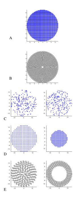
Figure 1. Arrays studied in this paper (dimensions are given in units of  $\lambda$ ): (a) squared pattern array with  $\lambda /2$  interspacing, (b) segmented annular array (SAA) with  $\lambda$  interspacing, (C) random sparse R-T arrays (C), vernier sparse R-T arrays (D), R-T vernier sparse from SAA
