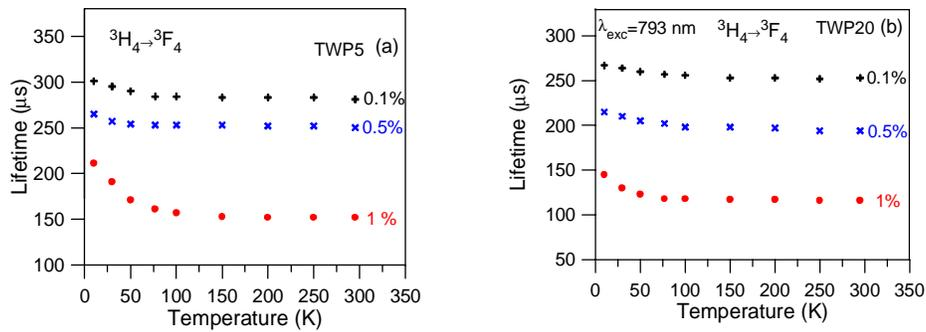
Fig. 5. Temperature dependence of the  ${}^3\text{H}_4$  level lifetime for different  $\text{Tm}_2\text{O}_3$  concentrations in TWP5 (a) and TWP20 (b) glasses.
