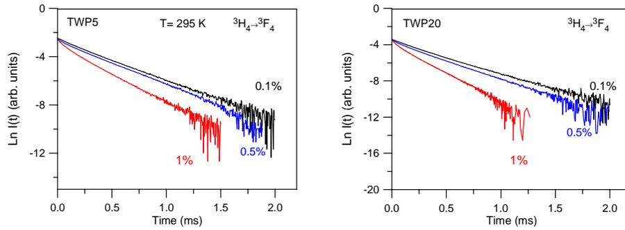
Fig. 4. Logarithmic plot of the fluorescence decay of the  ${}^3\text{H}_4$  level obtained under excitation at 793 nm at room temperature for TWP5 and TWP20 glasses doped with 0.1, 0.5, and 1 wt%.
