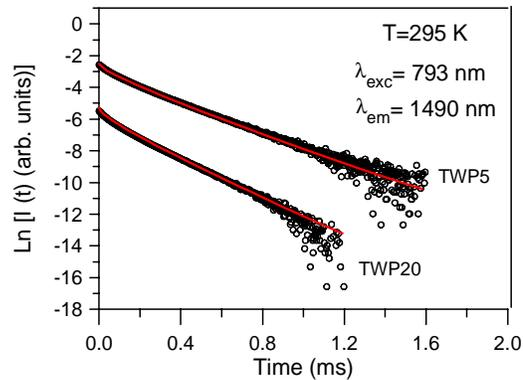
Fig. 6. Experimental emission decay curves of level  $^3\text{H}_4$  for TWP5 and TWP20 glasses doped with 1 wt%  $\text{Tm}_2\text{O}_3$  at room temperature and the calculated fit with Eq. (5) (solid line).
