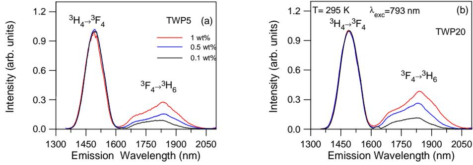
Fig. 2. Room temperature emission spectra of  $\text{Tm}^{3+}$  in TWP5 (a) and TWP20 (b) glasses for three  $\text{Tm}_2\text{O}_3$  different concentrations.
