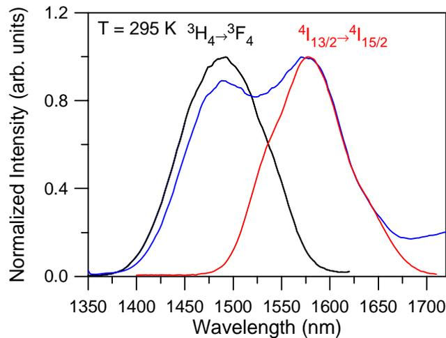
Fig. 3. Spectral overlap between the  ${}^3\text{H}_4 \rightarrow {}^3\text{F}_4$  (black) and  ${}^4\text{I}_{13/2} \rightarrow {}^4\text{I}_{15/2}$  (red) normalized emissions of  $\text{Tm}^{3+}$  and  $\text{Er}^{3+}$  ions respectively in TWP20 glass together with the emission spectrum of a codoped sample (blue).
