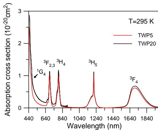
Fig. 1. Room temperature absorption cross-section of  $\text{Tm}^{3+}$  in TWP5 and TWP20 glasses.
