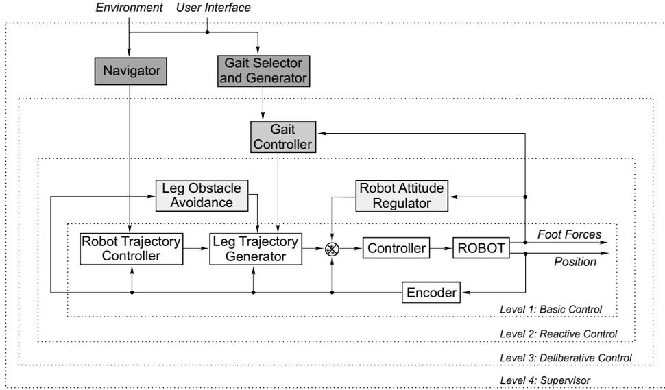
**Fig. 2 The SILO6 control architecture**
