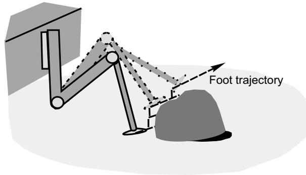
**Fig. 3 Foot trajectory during obstacle avoidance**
