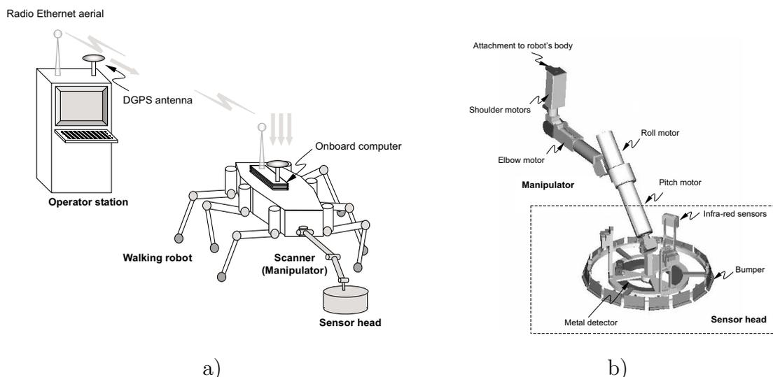
Fig. 1 a) Demining system; b) Scanning manipulator and sensor head
