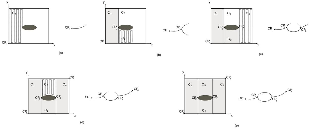
**Fig. 4 Incremental cellular decomposition and Reeb graph construction**
