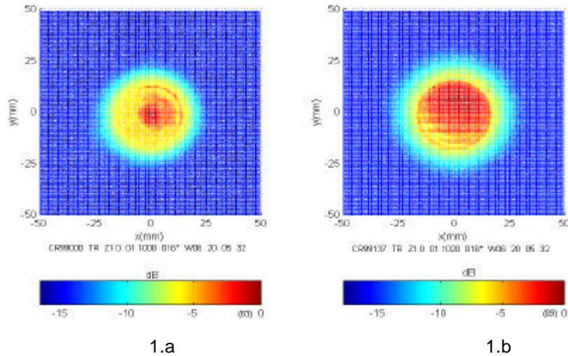
Figure 1. Transversal patterns measured near to the emitting surface ( $z = 1$  mm) for the 1 MHz, 34 mm in diameter applicators: a) - LOT 99000; b) LOT 99137
