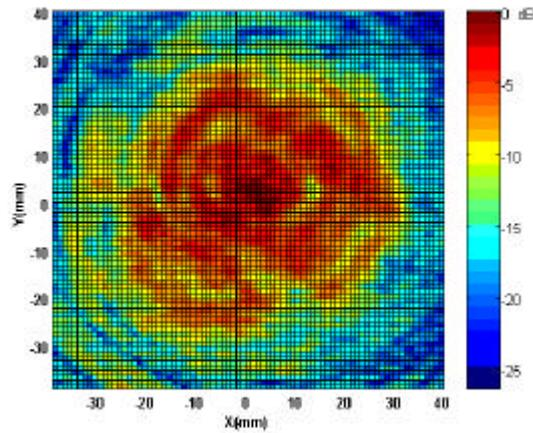
Figure 4. Transversal pattern measured at  $z = 3$  mm from the applicator Rich Mar V
