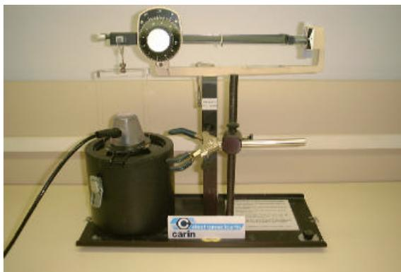
Figure 3. Radiation Force Balance
