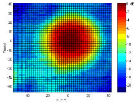
Figure 5. Transversal pattern measured at  $z = 233$  mm for the same applicator of Figure 4
