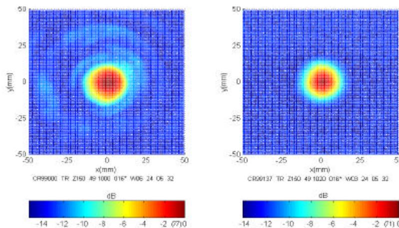
Figure 2. Transversal patterns measured at  $z = 150$  mm for the same applicators of Figure 1.
