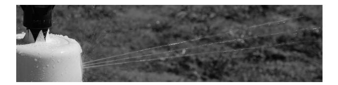
Figure 3. Three coherent jets emitted by three grooves of the FSPS 1P. A plastic screen has been installed to allow visualization of the jet shapes. The observed splash droplets, produced by the plastic screen, never reached the photographic area.
