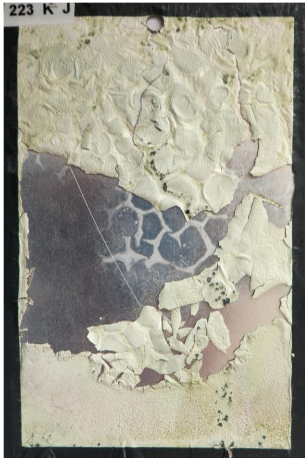
Figure 8 Appearance of the HT-V (15%) primer after 120h of exposure to the Kesternich test, showing significant delamination.
