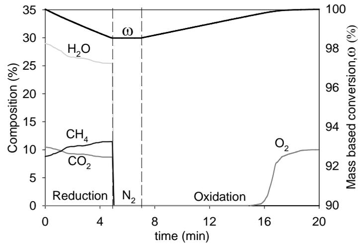
**Figure 4.** Product gas distribution in wet basis during reduction with CH<sub>4</sub> and subsequent oxidation for the 20<sup>th</sup> cycle. Reducing gas: 25% CH<sub>4</sub> + 20% H<sub>2</sub>O. T = 1173 K. N<sub>2</sub> to balance. Oxidation: 10% O<sub>2</sub>.
