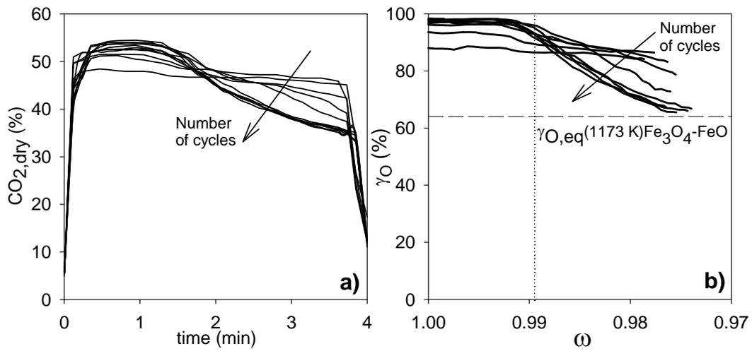
**Figure 7.** a) CO<sub>2</sub> dry basis profiles in the product gas for various reduction periods and b) Oxygen yield,  $\gamma_O$ , variation with the ilmenite mass based conversion for the reduction periods 3, 10, 20, 40, 50, 70, 85, and 100 for a 100 redox cycle test using syngas as reducing agent. Reducing gas: 21.5% H<sub>2</sub> + 28.5% CO + 8% H<sub>2</sub>O + 8.2% CO<sub>2</sub>. T = 1173 K.
