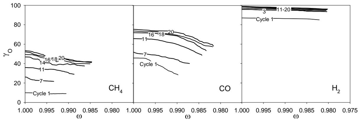
**Figure 5.** Oxygen yield,  $\gamma_{\text{O}}$ , as a function of the ilmenite mass based conversion,  $\omega$ , for the reduction period after 20 redox cycles for reduction with  $\text{CH}_4$  (Reducing gas: 25%  $\text{CH}_4$  + 20%  $\text{H}_2\text{O}$ ),  $\text{CO}$  (Reducing gas: 50%  $\text{CO}$  + 20%  $\text{CO}_2$ ) and  $\text{H}_2$  (Reducing gas: 50%  $\text{H}_2$  + 20%  $\text{H}_2\text{O}$ ).  $T = 1173 \text{ K}$ .
