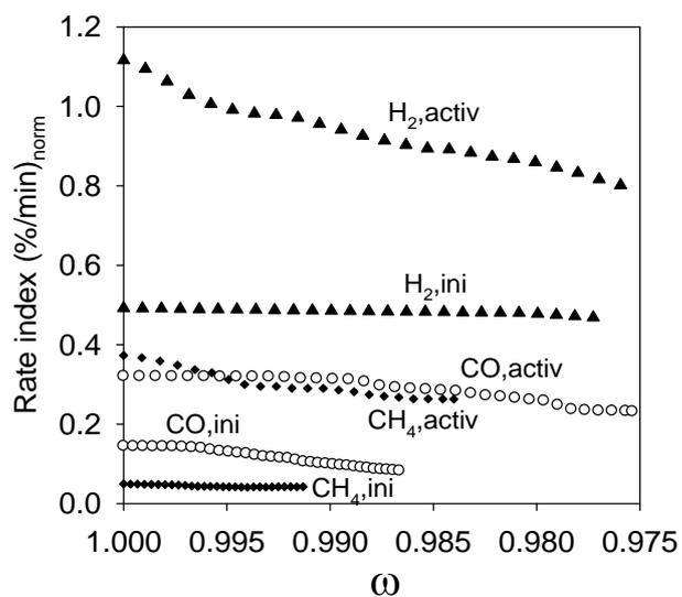
**Figure 6.** Normalized rate index as a function of the ilmenite mass based conversion,  $\omega$ , for the reduction reactions with CH<sub>4</sub>, CO and H<sub>2</sub> with calcined and activated ilmenite.  $P_{\text{ref}} = 0.15$ .  $T = 1173$  K.
