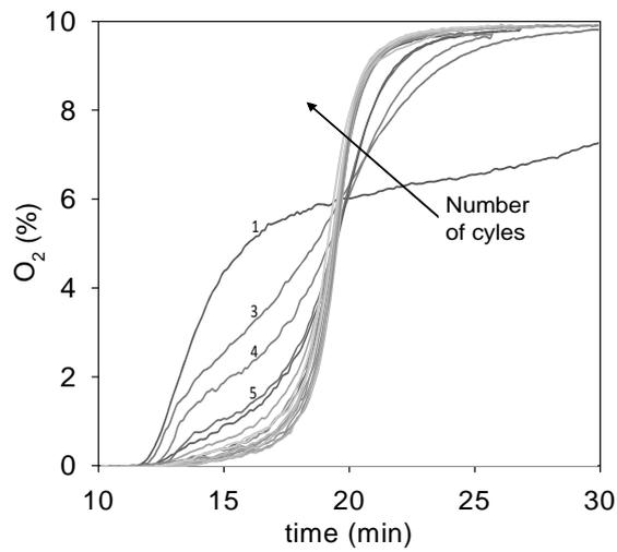
**Figure 9.** O<sub>2</sub> profiles in the product gas for the first subsequent 20 oxidation periods in a 100 redox cycle test. Previous reducing period of 4 minutes (Reducing gas: 21.5% H<sub>2</sub> + 28.5% CO + 8% H<sub>2</sub>O + 8.2% CO<sub>2</sub>) and purge with N<sub>2</sub> of 2 minutes. Oxidation with 10% O<sub>2</sub> and gas velocity: 23 cm/s. T = 1173 K. The initial solid mass based conversion of the partially reduced ilmenite was about 0.975.
