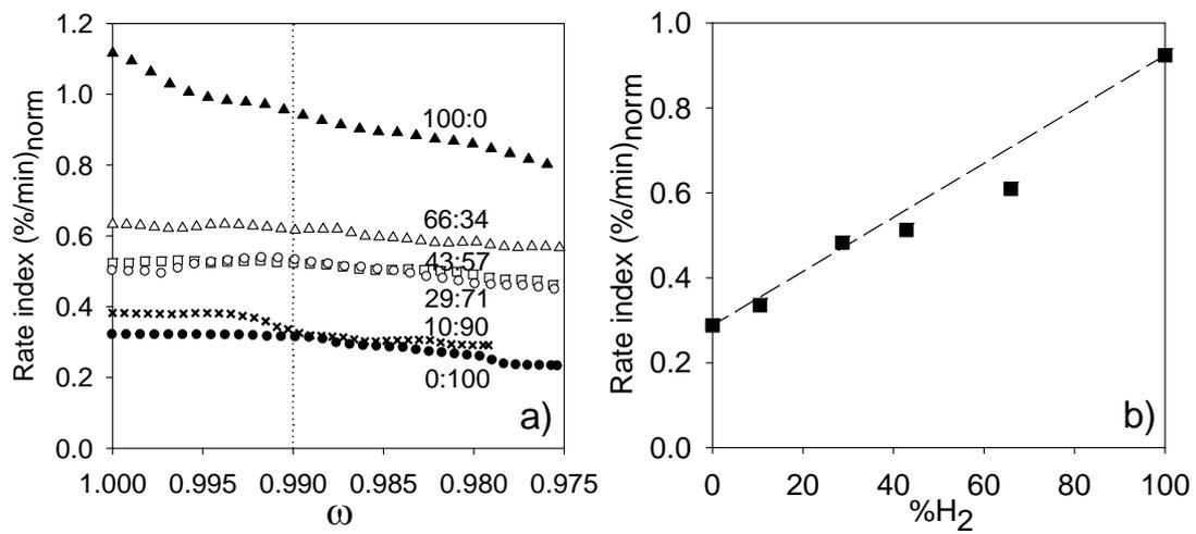
**Figure 8.** a) Normalized rate index variation along the reducing cycle as a function of ilmenite mass based conversion and b) Average normalized rate index as function of the fraction of H<sub>2</sub> in the reducing gas for different H<sub>2</sub>:CO mixtures tested (see conditions in Table 2). T = 1173 K.
