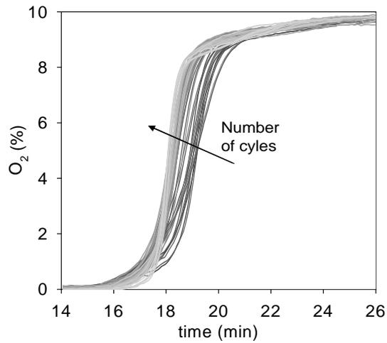
**Figure 10.** O<sub>2</sub> profile evolution in the product gas for the oxidation period from cycle 20 to cycle 100 Previous reducing period of 4 minutes (Reducing gas: 21.5% H<sub>2</sub> + 28.5% CO + 8% H<sub>2</sub>O + 8.2% CO<sub>2</sub>) and purge with N<sub>2</sub> of 2 minutes. Oxidation with 10% O<sub>2</sub> and gas velocity: 23 cm/s. T = 1173 K. The initial conversion  $\omega$  of the partially reduced ilmenite was about 0.975.
