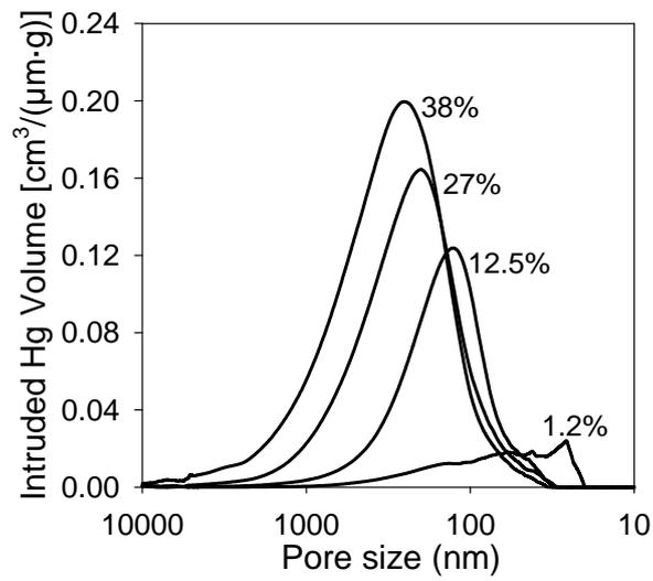
**Figure 11.** Pore distribution of different samples of ilmenite: Calcined with porosity of 1.2%, after 8 cycles, with porosity of 12.5%, after 18 cycles with porosity of 27% and after 100 cycles with porosity of 38%. Ilmenite samples taken after several redox cycles in Batch Fluidized Bed. Reductions with syngas as fuel (see conditions in Table 2). T = 1173K.
