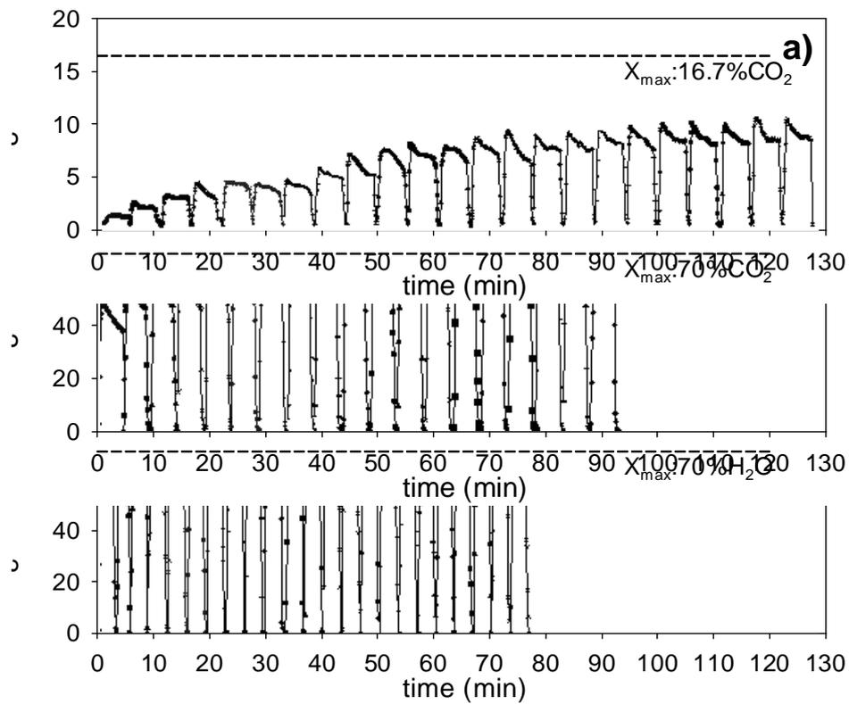
**Figure 3.** Profiles of CO<sub>2</sub> or H<sub>2</sub>O fractions in the product gas (wet basis) during consecutive reduction periods, for a) CH<sub>4</sub>, b) CO and c) H<sub>2</sub> as reducing gases. The intervals between reducing periods have been removed.  $X_{\max}$  is the maximum CO<sub>2</sub> or H<sub>2</sub>O corresponding fraction if full combustion was reached. Experimental conditions are showed in Table 2. T = 1173 K.
