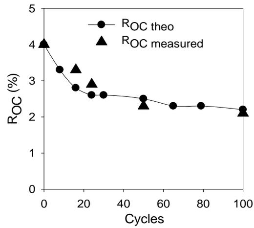
**Figure 14.** Measured and theoretical  $R_{OC}$ .  $R_{OC}$  variation with the number of cycles reduction periods 3, 10, 20, 40, 50, 70, 85, and 100 in a 100 redox cycle test using  $H_2+CO$  syngas as reducing agent. Reducing gas: 21.5%  $H_2$  + 28.5%  $CO$  + 8%  $H_2O$  + 8.2%  $CO_2$ .  $T = 1173$  K.
