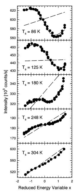
FIG. 2. Examples of the fit of the experimental line shapes (dots) by the F(x) function (solid line) defined by Eq. (7) with the variable x given by Eq. (6). The dashed lines show the linear background term  $\alpha + \beta x$ . At the surface temperatures  $T_s = 86$ , 125, and 180 K two critical points are visible, while at  $T_s = 248$  K only one is visible. At  $T_s = 304$  K no critical points are observed.
