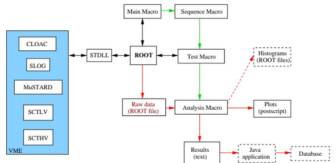
Fig. 2. Schematic diagram of the SCTDAQ system.
