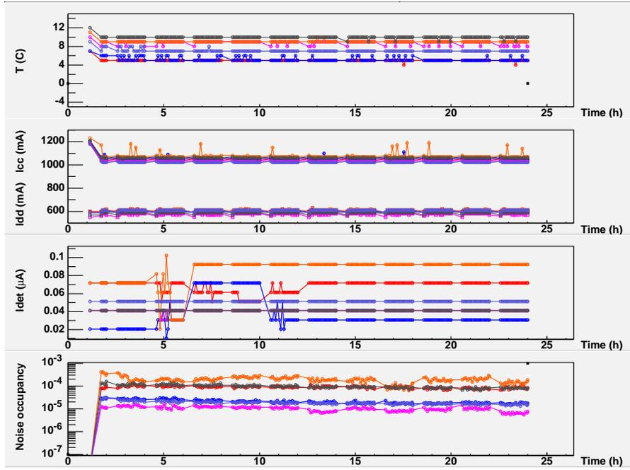
Fig. 5. Long-term test results for six modules showing from top to bottom: hybrid temperature; analog ( $I_{cc}$ ) and digital ( $I_{dd}$ ) current; detector leakage current ( $I_{det}$ ); and noise occupancy as a function of time.
