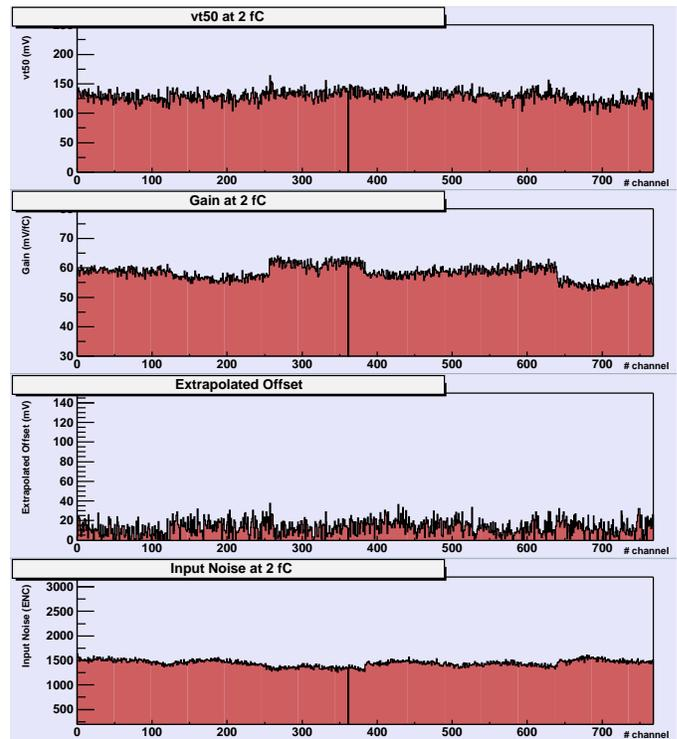
Fig. 4. Typical set of plots obtained with the Response Curve procedure before trimming and for one data stream, corresponding to six chips (768 channels). From top to bottom the  $vt_{50}$  value, the gain, the offset and the input noise are shown for each channel.
