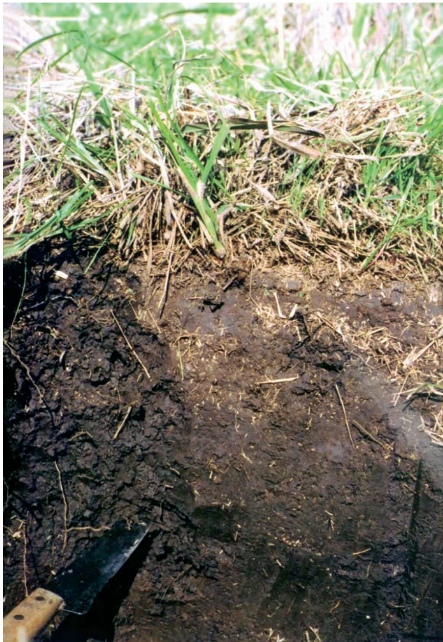
Fig. 9.3 Topsoil of Ramallo series soil, under natural conditions. The A1 horizon has a depth of 31 cm, and an organic matter content of 4.27%
