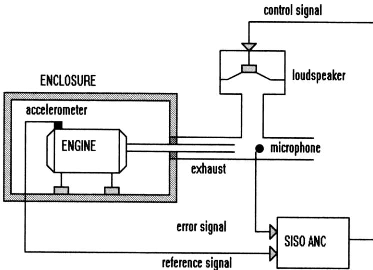
FIGURE 2. Setup of the passive/active control system
