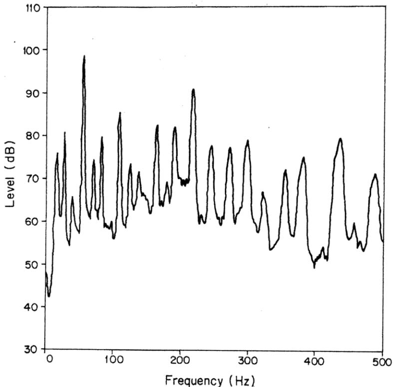
FIGURE 3. Reference signal supplied by an accelerometer over the air filter case of the generator
