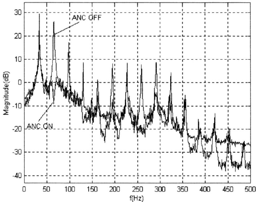
**FIGURE 4.** Averaged log-magnitude spectra of the exhaust noise with and without cancellation
