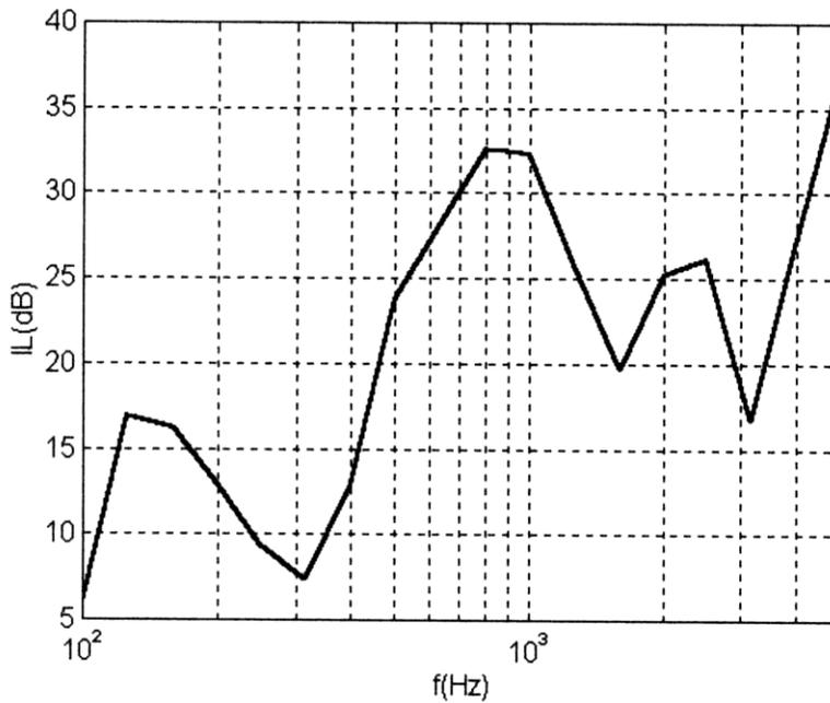
FIGURE 1. Insertion Loss of the passive enclosure
