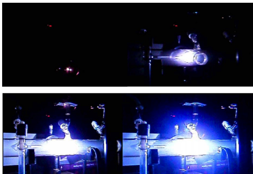
Figure 2. Four images of the laser-induced breakdown of nitrogen at atmospheric pressure at different times of the experiment.
