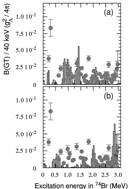
FIG. 4. Experimental Gamow-Teller strength distribution measured for  $^{74}\text{Kr}$  (filled circles) compared to self-consistent HF calculations [39,41] assuming for the  $^{74}\text{Kr}$  ground state (a) an oblate ( $\beta_0 = -0.15$ ) shape, and (b) a prolate ( $\beta_0 = +0.39$ ) shape. The calculations were performed using the SG2 Skyrme interaction.
