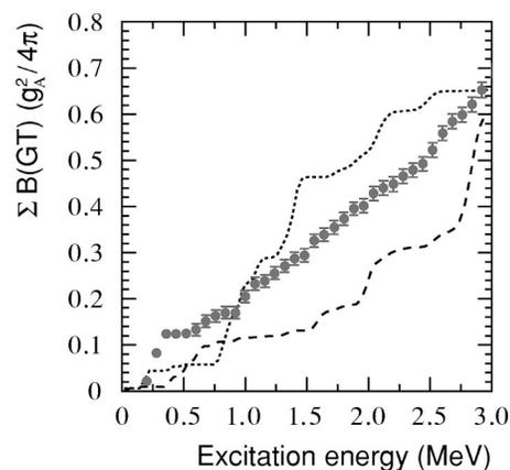
FIG. 5. Accumulated GT strength in  $^{74}\text{Kr}$  as a function of the excitation energy of the daughter nucleus. The dotted and dashed lines correspond to the oblate and prolate solutions of HF calculations using the SG2 interaction, respectively.
