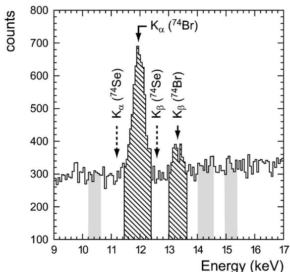
FIG. 2. X-ray spectrum obtained with the germanium planar detector and showing the  $K_{\alpha}$  and  $K_{\beta}$  transitions in  $^{74}\text{Br}$ . The expected positions of the  $K_{\alpha}$  and  $K_{\beta}$  transitions in  $^{74}\text{Se}$  are also shown. The shaded areas show the energy gates used for background subtraction.
