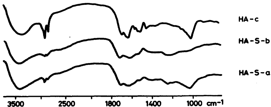
Fig. 1. IR spectra of the humic acids before (HA-S-b) and after (HA-S-a) the compost treatment, and from compost (HA-C).
