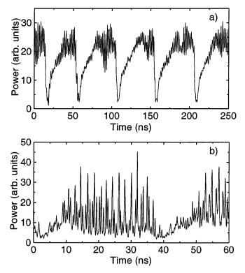
FIG. 1. Total intensity as a function of time taken with (a) the oscilloscope, and (b) the streak camera with a time resolution of about 230 ps. Note the pseudoperiodicity of the signal at the round-trip time in the external cavity ( $\sim 2$  ns).
