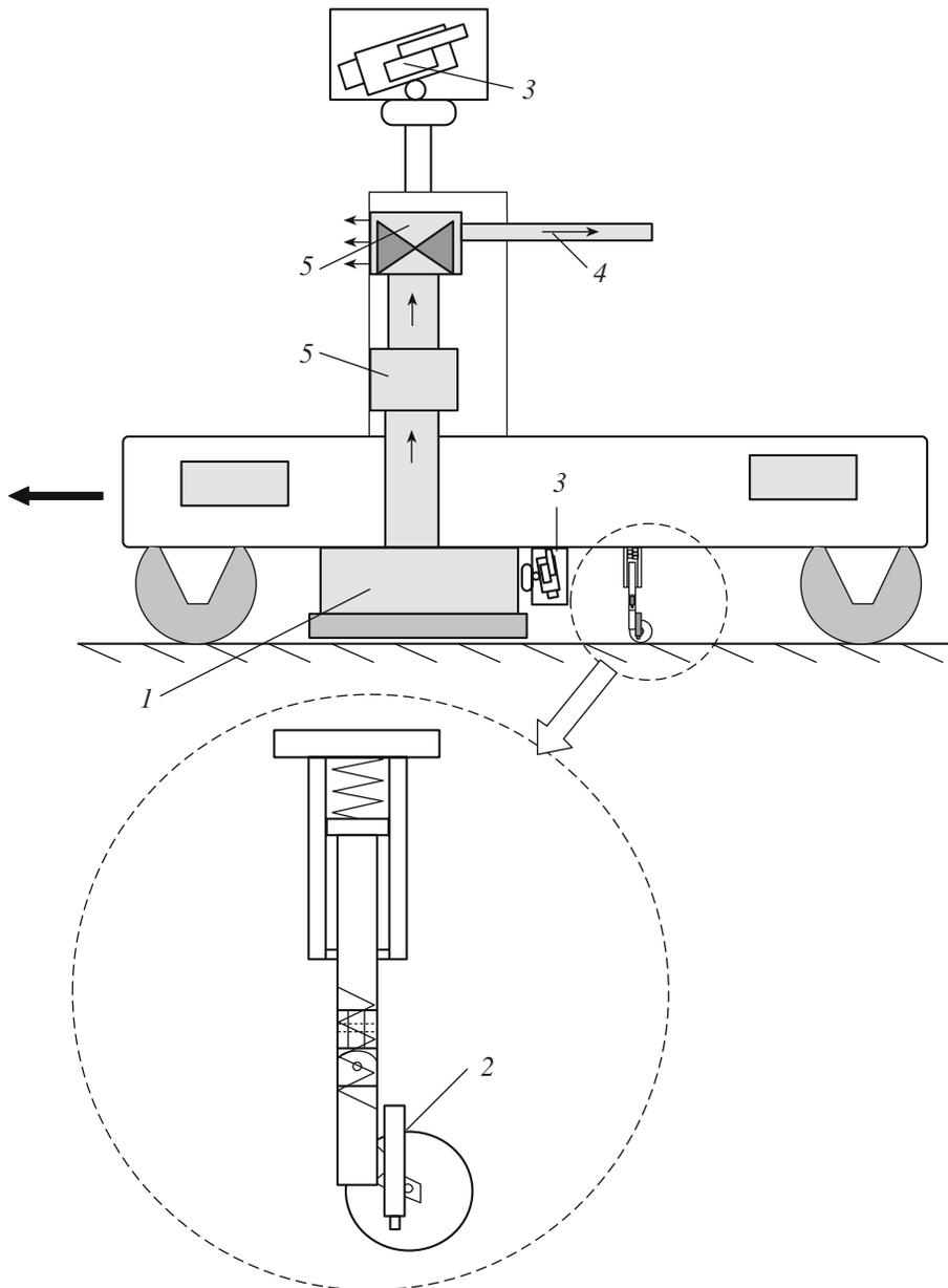
Fig. 7. Scheme of the underwater robot and device for testing the sheet thickness containing elements for its fixation: (1) cleaning brush with a fence; (2) ultrasonic probe; (3) rotating video camera; (4) tubes and cables connecting the robot with the above-water equipment; (5) technological equipment (pump, grinder, filter-separator, etc).
