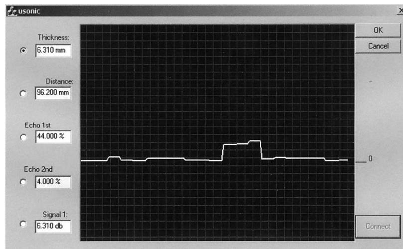
**Fig. 9.** Information on the sheet thickness of the ship's hull displayed on the operator's screen during the robot movement.
