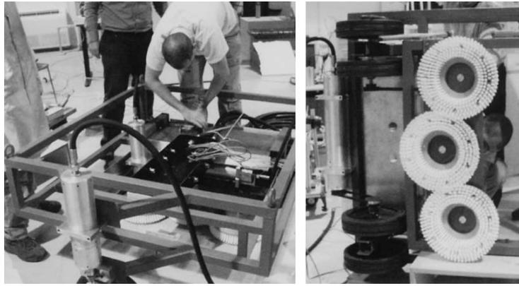
**Fig. 8.** Assembling of the AURORA underwater robot.
