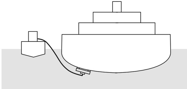
Fig. 2. Schematic view of interaction of the robot with a tested ship.
