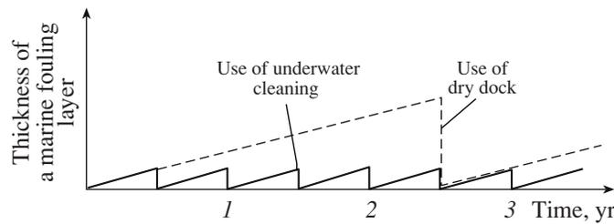
Fig. 1. Time dependence of thickness of a marine fouling layer.
