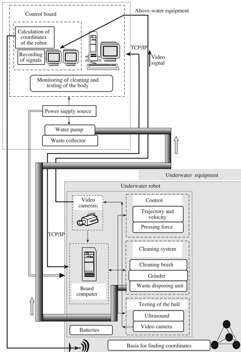
Fig. 3. Structure of above-water and underwater parts of the system.
