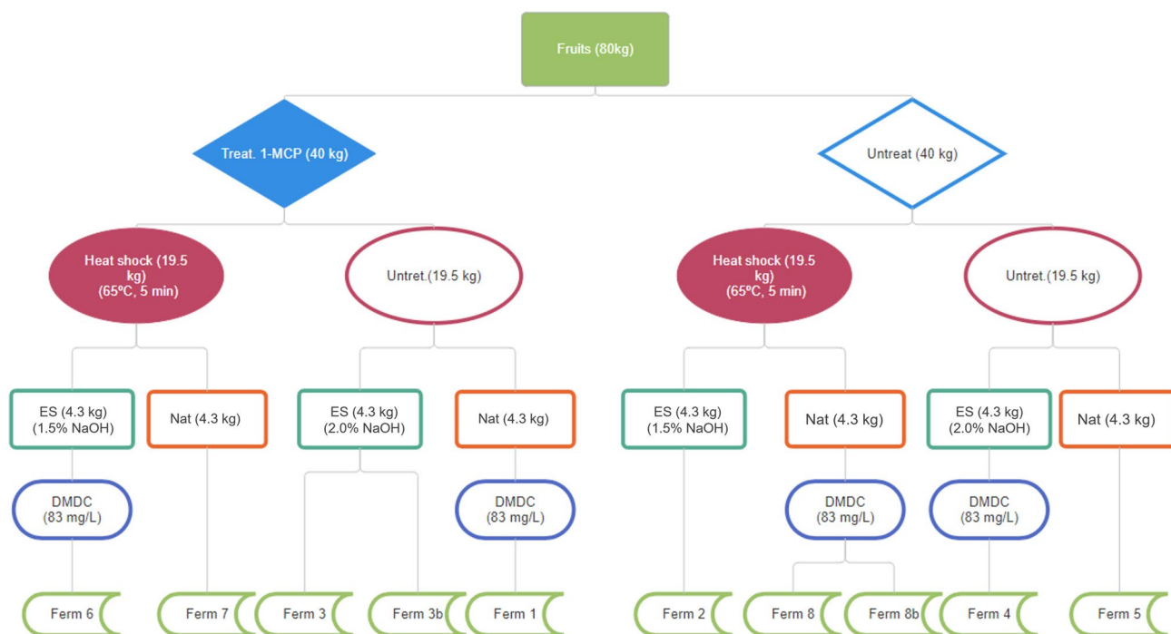
Fig. 1 Scheme of the experimental design used in this work, displaying the various processing steps and treatments administered to each fermenter container. A summarized version for statistical analysis can also be found in Table S1 (Supplementary Material)
