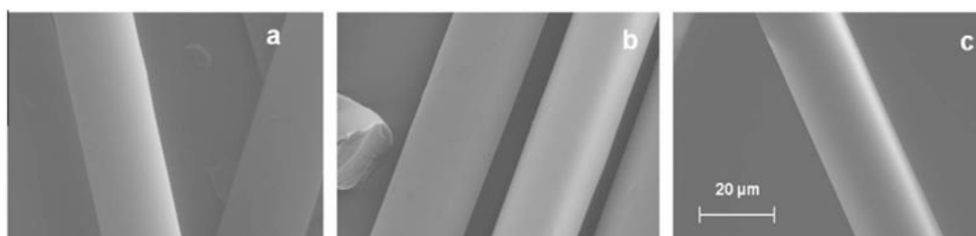
Fig. 2. Scanning electron micrographs of green carbon fibres obtained from (a) AOP1, (b) AOP2 and (c) AOP3.
