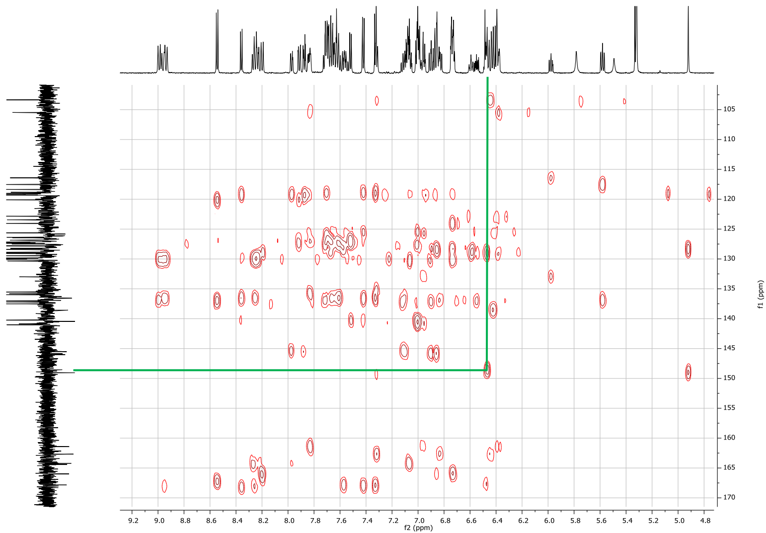
Figure S32. HMBC ^1\text{H} - ^{13}\text{C}\{^1\text{H}\} NMR spectrum (125 MHz, \text{CD}_2\text{Cl}_2 , 298 K) of complex 9 .
