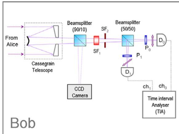
Figure 3. Bob's module.  $SF_1$  and  $SF_2$  are a set of spectral filters and a spatial filter, respectively;  $P_0$  and  $P_1$  are two high extinction-ratio polarisers;  $M_1$  is a high-reflectivity mirror; and  $D_0$  and  $D_1$  are single-photon detectors.
