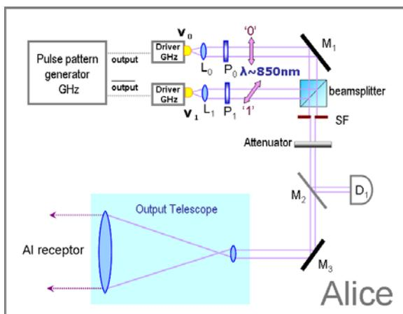
Figure 2. Alice's module.  $V_0$  and  $V_1$  are two VCSELs;  $L_0$  and  $L_1$  are two optical lenses;  $P_0$  and  $P_1$  are two high extinction-ratio polarisers;  $M_1$ ,  $M_2$  and  $M_3$  are three high-reflectivity mirrors; and SF is a spatial filter.
