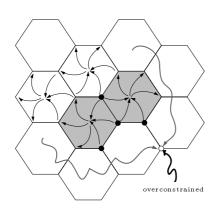
Fig. 3. A height propagation starting at four pre-specified (bold) vertices. Several vertices can have an overconstrained height.
