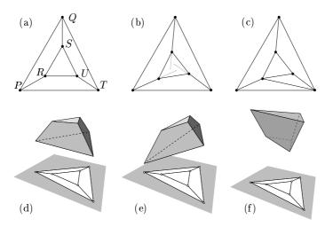
**Fig. 2.** A truncated tetrahedron (a) and three possible reconstructions (d, e, f). The slightest perturbation destroys the correctness of the projection (b), but this can be avoided adding new triangular faces (c).
