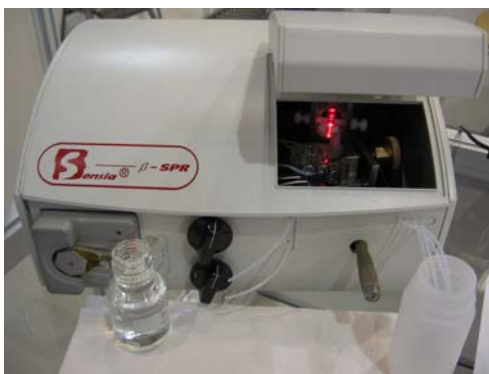
Fig 2. Portable SPR platform, including sensor, optics, electronics and flow delivery system.
