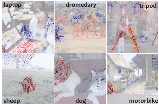
Figure 1. Illustration of our proposed method for attribution map generation. Given an input image, we want to obtain a score for each pixel estimating their contribution to the CNN output for a target label (in bold). Our approach is able to identify discriminative image pixels that contribute positively (red) or negatively (blue) to the prediction, and pixels corresponding to nuisance factors that have no effect on the output (white). For instance, in bottom-middle, positive attributions are assigned to the dog whereas negative scores correspond to pixels belonging to the cat. Additionally, no attributions are assigned to the non-discriminative background pixels. The disentanglement of this components produces fine-grained pixel-level attributions revealing the patterns used by the network during inference. We show that the generated attribution maps are more informative and visually interpretable than the ones obtained by previous methods.
