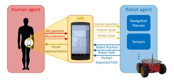
Fig. 2. **Information flow considered in our proposal.** Smartphone acts as an HRI interface converting graphic information understandable by the human into messages understandable by the robot and vice versa.
