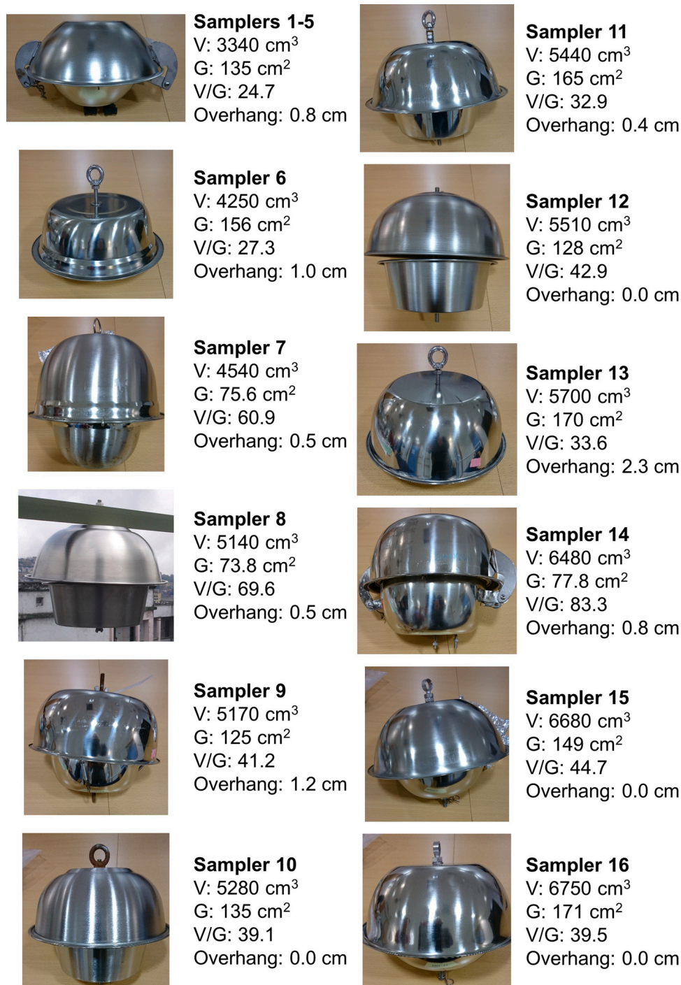
Fig. 1. Sampler designs used in the study and their basic dimensions. V indicates volume, G indicates the area of the horizontal gap between upper and lower dome, V/G is the ratio of the dome volume to gap area, and overhang is the distance the upper dome extends over the lower dome.
