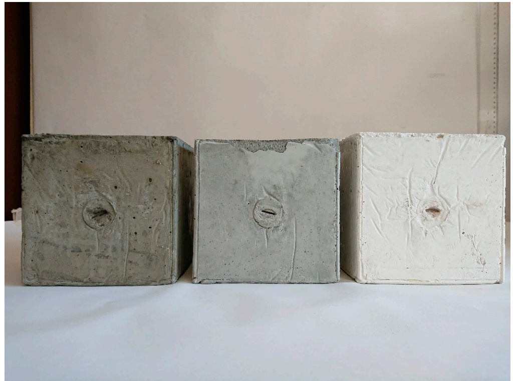
Figure 3. Cubic specimens of the binders 100FA (left), 50FA50WG (centre) and 100WG (right), showing the insertion points of the bender elements which used to measure the seismic waves.
