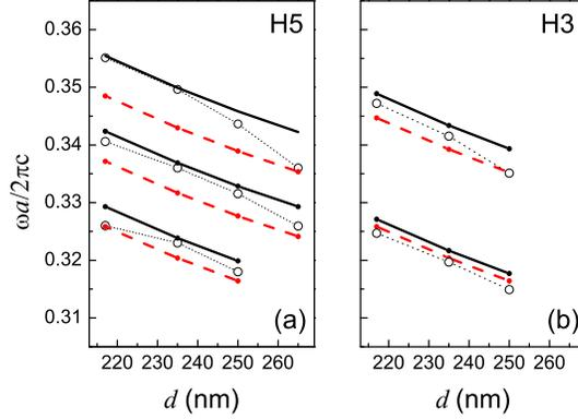
FIG. 5: (color online) Normalized frequencies of emission peaks produced by localized modes in H5 (a) and H3 (b) microcavities as a function of InP layer thickness,  $d$ . Open circles represent the experimental data obtained by microphotoluminescence. The dotted lines are guides for the eye. Solid (red dashed) lines show the theoretical prediction given by the model of confined triangular-symmetry (hexagonal-symmetry) modes.
