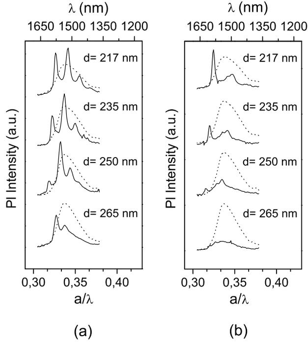
FIG. 4: Photoluminescence spectra of the H5 (a) and H3 (b) microcavities with different slab thicknesses  $d$  (solid lines). The spectra of an unpatterned region in the vicinity of the microcavity is also shown (dotted lines). Here  $\lambda$  is the vacuum wavelength:  $a/\lambda = \omega a / 2\pi c$ .
