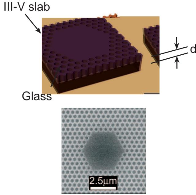
FIG. 1: (Lower image) Scanning electron microscopy image of the fabricated H5 cavities. (Upper image) Schematic view of H5 microcavity fabricated on the III-V semiconductor slab with a thickness  $d=265$  nm bonded to a glass substrate.
