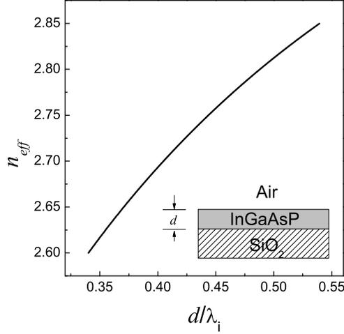
FIG. 3: Effective refractive index  $n_{eff}$  versus InGaAsP layer thickness over internal wavelength  $d/\lambda_i$  in a planar waveguide with  $\epsilon_f = 10.89$  (InGaAsP),  $\epsilon_s = 2.34$  (SiO<sub>2</sub>) and  $\epsilon_t = 1$  (air).
