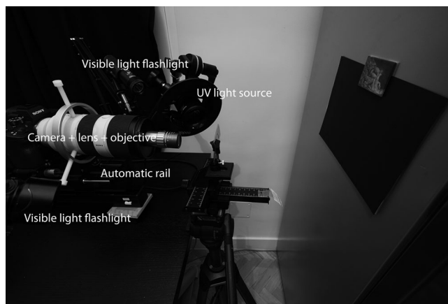
FIGURE 1 Setup used for the acquisition of extended depth of focus (EDF) images under visible or UV illumination
