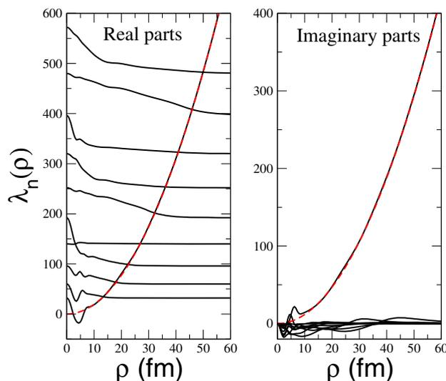
**Figure 1.** The 10 real and imaginary angular eigenvalues as function of  $\rho$  for  $0^+$  for three bosons interacting by  $d$ -waves. The two-body systems have a  $d$ -resonance at 4.53 MeV with a width of 2.36 MeV ( $\theta_R = 0.127$ ). The red curves are the real and imaginary parts of the parabola  $2m|E|\rho^2 \exp(2i(\theta - \theta_R)) / \hbar^2$ . The complex scaling angle  $\theta = 0.4$ .
