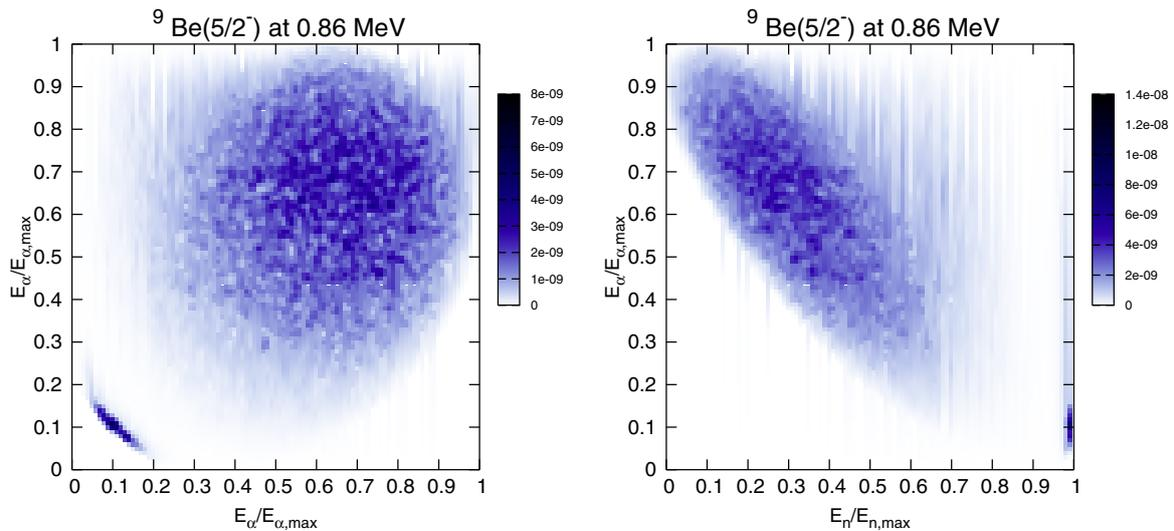
**Figure 5.** The computed probability distribution for finding one  $\alpha$ -particle energy when another  $\alpha$ -particle (left) or a neutron (right) already has a given value.
