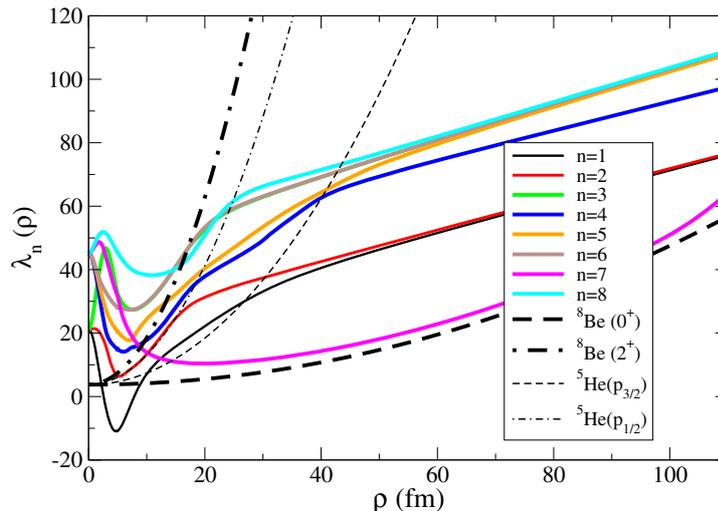
**Figure 2.** The real part of the lowest angular eigenvalues for the  ${}^9\text{Be}(5/2^-)$ -resonance. The thick and thin dashed parabolic curves are the asymptotics corresponding to the lowest  $(0^+, 2^+)$  and  $(p_{3/2}, p_{1/2})$  resonances for  ${}^8\text{Be}$  and  ${}^5\text{He}$ , respectively.
