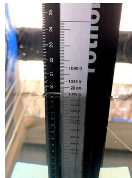
Figure 4. Measurement of volume of evaporated water.
