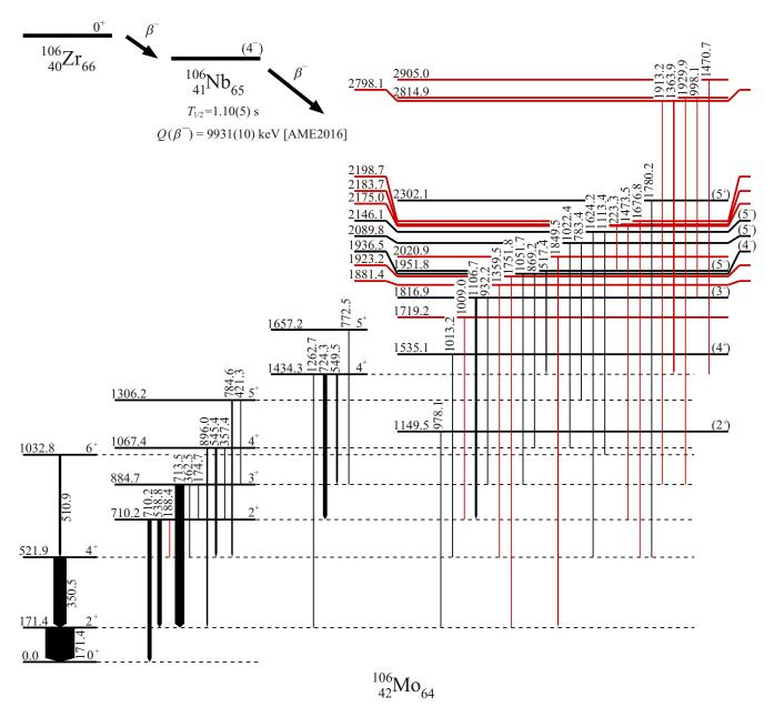
FIG. 2. The proposed level scheme of <sup>106</sup>Mo obtained from the  $\beta$ -decay chain <sup>106</sup>Zr  $\rightarrow$  <sup>106</sup>Nb  $\rightarrow$  <sup>106</sup>Mo. The  $Q(\beta^{-})$  of <sup>106</sup>Nb is taken from the atomic mass evaluation (AME2016 [33]). The arrow width is proportional to the relative intensity  $I_{\gamma}$  (Zr  $\rightarrow$  Mo, given in Table II). Red lines are the new levels and transitions. Spin parities of the known states are taken from ENSDF [34].
