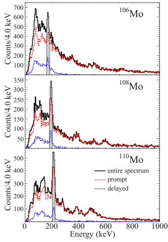
FIG. 9. The  $\gamma$ -ray energy spectra of the LaBr<sub>3</sub>(Ce) array. The energy region used to make the time spectra of Fig. 8 are highlighted with gray. The prompt,  $|\Delta T| < 1$  ns, and delayed,  $\Delta T > 1$  ns, components are shown by the red and blue dotted lines, respectively.
