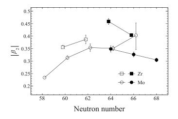
FIG. 11. Quadrupole deformation parameter  $\beta$  for Zr (square) and Mo (circle) isotopes. Filled circles are the present results for the Mo isotopes. Filled squares for the Zr isotopes are the results from the same data set [53], but the values were recalculated from  $B(E2; 2_1^+ \rightarrow 0_1^+)$  by using the formula given in the review paper [48]. Open circles and squares are taken from the review paper [48] and a later work [54].
