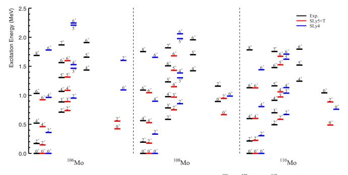
FIG. 17. The experimental and theoretical energies of the low-lying excited states in  $^{106}$ Mo,  $^{108}$ Mo, and  $^{110}$ Mo. Black lines present the experimental results, and red and blue lines present the results from the theoretical calculations using SLy5 + T and SLy4, respectively.
