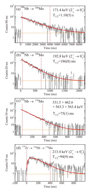
FIG. 3. The time spectra of  $\beta$ -delayed  $\gamma$  rays in the Mo isotopes. Dashed lines indicate the fitting region of the decay curve to determine the  $\beta$ -decay half-life,  $T_{1/2}$ . Orange lines are the constant background, which was determined by fitting to the negative-time region. The  $\beta$ -delayed  $\gamma$  rays with 531.5, 462.6, 563.3, and 563.4 keV from the implanted <sup>110</sup>Nb were selected as the  $\beta$  decays of the high-spin state in <sup>110</sup>Nb.
