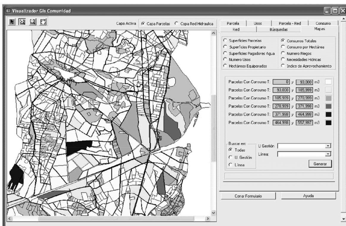
Fig. 3. GIS interface to Ador, showing a graduated colour map of water use per cadastral plot. Other options permit to display land ownership, types of water uses or the hierarchy of the conveyance network.
