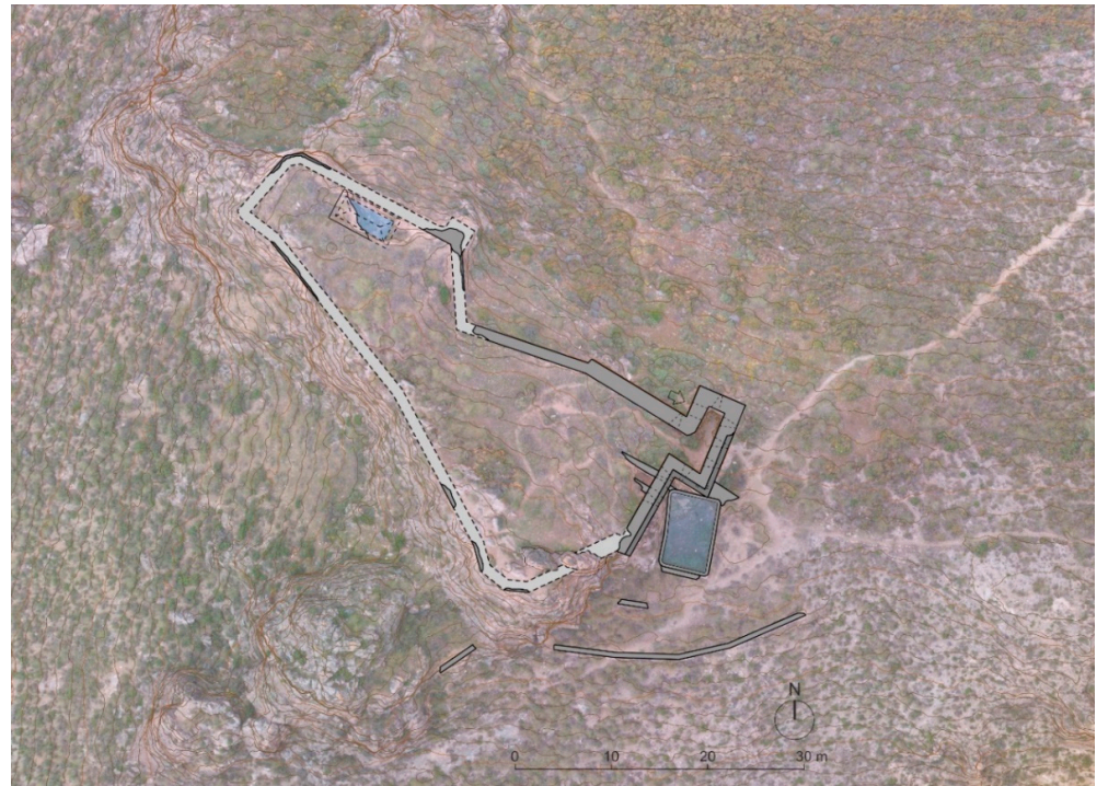
Figure 4. Plan of Mondújar Castle. The dark grey parts correspond to the structures preserved, and the light grey ones are the parts that have disappeared. We also present the outside cistern, the vestiges of the interior one and walls of the exterior terraces (A. Orihuela; V. Martín-Madrid, 2020).
