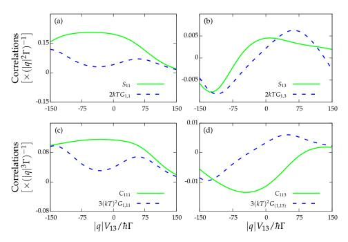
**Figure 6.** Fluctuation–dissipation theorem in a non-stalled configuration  $I_1 \neq 0$  and  $J_1 \neq 0$  for: (**a**) the drag current; and (**b**) the drag and drive currents. Fluctuation–dissipation relations in a non-stalled configuration  $I_1 \neq 0$  and  $J_1 \neq 0$  for: (**c**) the drag current; and (**d**) the drag and drive currents. The rest of the parameters are those of Figure 3.
