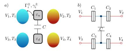
**Figure 1.** (a) Double quantum dot capacitively coupled to four terminals held at potentials  $V_i$  and temperatures  $T_i$ , for i = 1, 2, 3, 4. The transition rates  $\Gamma_i^{\pm}$  and  $\gamma_i^{\pm}$  for each barrier are described in the main text. (b) Electrostatic sketch showing the capacitors and voltages involved in the description of the energy levels of the quantum dots.
