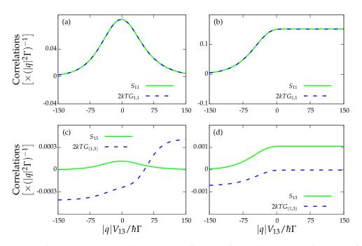
**Figure 4.** Fluctuation–dissipation theorem  $S_{\alpha\beta} = 2k_B T G_{(\alpha,\beta)}$  for: (**a**) the strong coupling regime for the drag current,  $I_1 = 0$  and  $J_1 = 0$ ; (**b**) the locally charge-stalled configuration,  $I_1 = 0$  and  $J_1 \neq 0$ ; and (**c**,**d**) the drag and drive currents with  $I_1 = 0$  and  $J_1 = 0$ , and  $I_1 = 0$  and  $J_1 \neq 0$ , respectively. The rest of the parameters are those of Figure 3.
