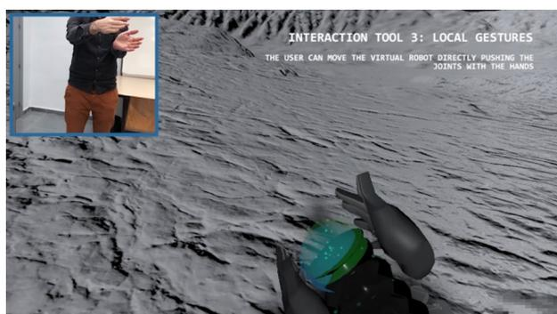
**Fig. 8** Local gestures strategy. The user's hands are tracked using a Leap Motion system so they can be used to directly interact with the virtual robot
