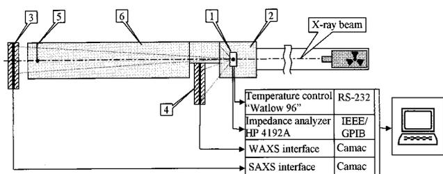
FIG. 4. Scheme of the experimental setup for simultaneous SAXS-WAXS-DS experiments at polymer beam line A2 at HASYLAB-DESY. (1) SAXS-WAXS-DS sample cell, (2) vacuum chamber, (3) SAXS detector, (4) WAXS detector, (5) Beam stop, and (6) vacuum evacuated optical path.
