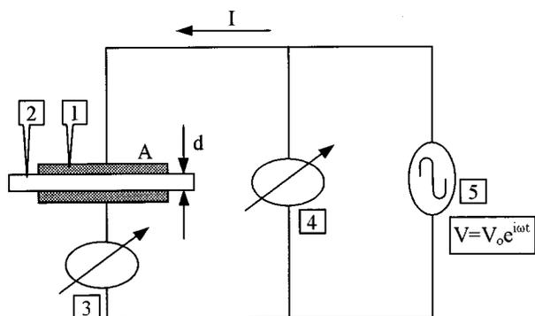
FIG. 1. Schematic view of a typical dielectric spectroscopy experiment. (1) Electrodes of area  $A$ , (2) sample film of thickness  $d$ , (3) current analyzer, (4) voltage analyzer, and (5) alternating voltage generator.
