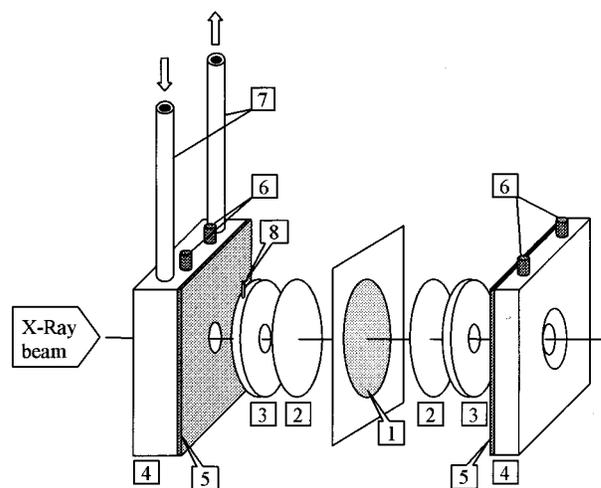
FIG. 3. Scheme of the SAXS-WAXS-DS cell. (1) Sample, (2) aluminum disks, (3) electrodes, (4) heating blocks, (5) insulating polyamide film, (6) heating elements, (7) cooling pipes, and (8) PT-100 thermometer.
