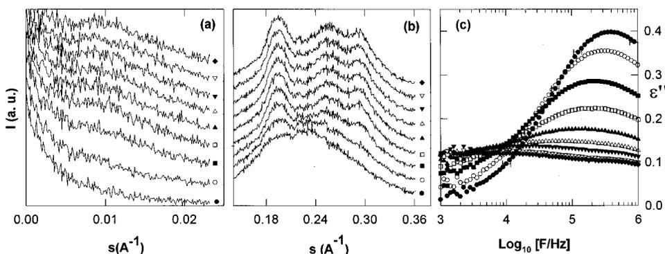
FIG. 5. Simultaneous SAXS (a), WAXS (b), and DS (c) experiment during crystallization of initially amorphous PET at  $T_c = 116^\circ\text{C}$ . Different symbols correspond to different crystallization times: (●)  $t_c = 1$ , (○)  $t_c = 5$ , (■)  $t_c = 10$ , (□)  $t_c = 15$ , (▲)  $t_c = 20$ , (△)  $t_c = 25$ , (▼)  $t_c = 30$ , (▽)  $t_c = 50$ , and (◆)  $t_c = 100$  min.
