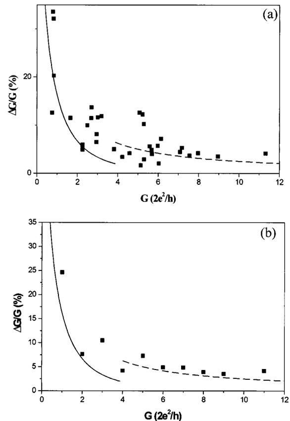
FIG. 1. (a) Experimental values of BMR for iron. The solid line is the calculation for theory developed in Ref. 2 for  $\zeta = 0.5$  and  $r = 3$  (from Ref. 7). The dashed line shows the  $\alpha/N$  behavior ( $\alpha = 25$ ) for  $N \gg 1$ . (b) The same as (a) but for the average experimental data. Notice that the BMR values are approximately ten times smaller for Fe than for Ni and Co (in Fig. 2).
