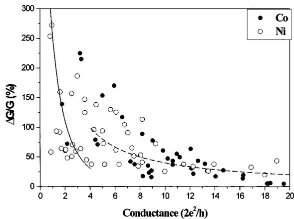
FIG. 2. Ballistic magnetoresistance for Ni and Co: the solid line is the calculation for  $\zeta=0.87$  and  $r=12$ ; the dashed line shows  $\alpha/N$  behavior ( $\alpha=400$ ). Data for comparison are from Refs. 1 and 2.
