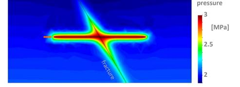
fluid pressure anisotropy due to existing fracture
