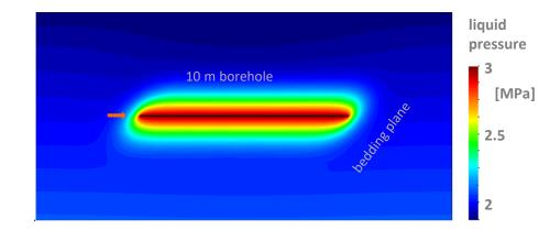
fluid pressure anisotropy due to bedding plane angle
