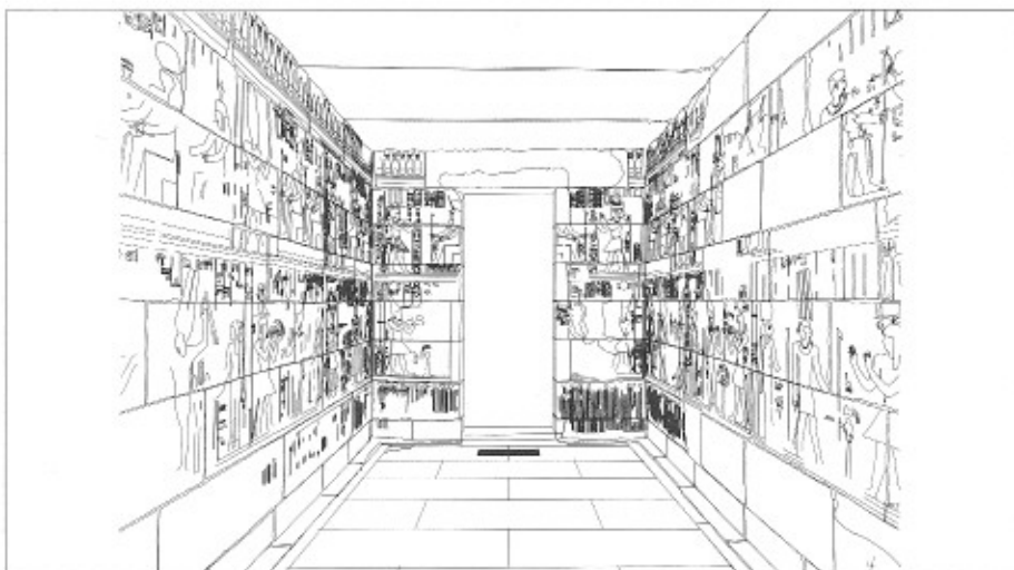
Fig. 4. Perspective of the decorated chamber of the Egyptian temple of Debod, Madrid, an example of a three-dimensional model produced from photogrammetry managed with CAD.
