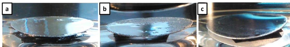
Figure 10. Pictures showing the appearance of the mirror on coatings prepared with P7 particles: (a) minutes after immersion, (b) after 100 h of immersion, and (c) after removing the water and filling the container again.
